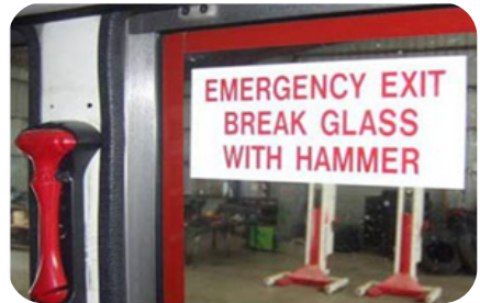
Internal emergency exit sign with a 20 mm wide contrasting band – lettering less than 75 mm high.
