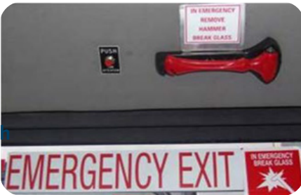
Internal sign and instructions with operating device (hammer). Note no coloured band required due to size of lettering.
