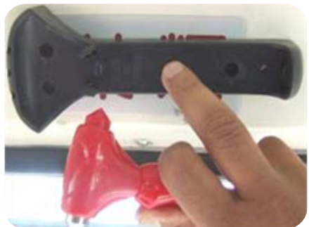
Glass breaking device - hammer - securely fitted next to the dedicated emergency exit.
