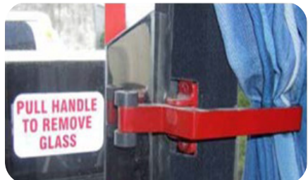
Internal emergency exit sign with a 20 mm wide contrasting band – lettering less than 75 mm high.
