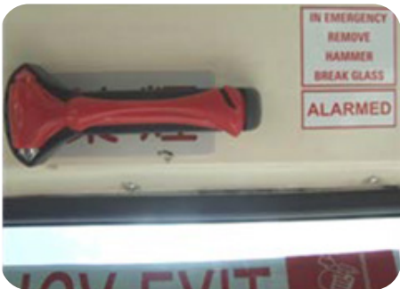
Glass breaking device - hammer - securely fitted next to the dedicated emergency exit.
