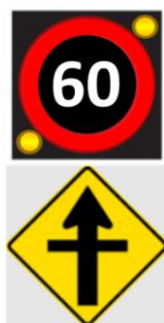
Figure 3 - Example of an AWRS (with pulsing roundel) with supplementary warning sign (PW-9 intersection layout static panel) (Source: Section 8.2 of ITS Design Standard: Active warning and regulatory signs).
