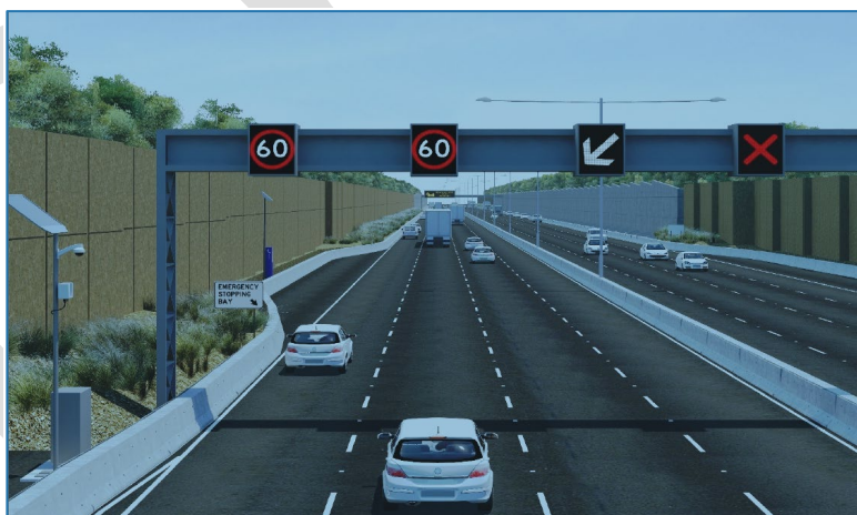
Figure 4. Integrated lane and speed management operating mode
