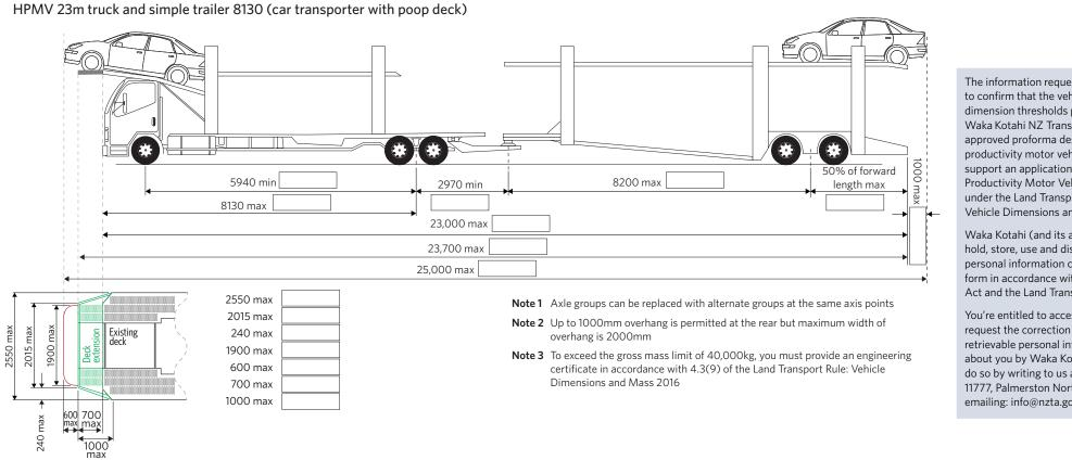
The information requested is required to confirm that the vehicle meets the dimension thresholds provided in Waka Kotahi NZ Transport Agencyapproved proforma designs for high productivity motor vehicles and to support an application for a High Productivity Motor Vehicle Permit under the Land Transport Rule: Vehicle Dimensions and Mass 2016.
