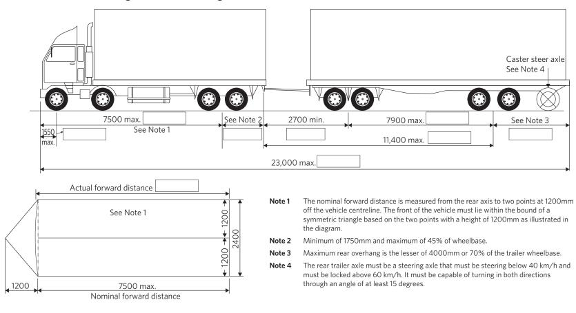
The information requested is required to confirm that the vehicle meets the dimension thresholds provided in Waka Kotahi NZ Transport Agencyapproved proforma designs for high productivity motor vehicles and to support an application for a High Productivity Motor Vehicle Permit under the Land Transport Rule: Vehicle Dimensions and Mass 2016.
