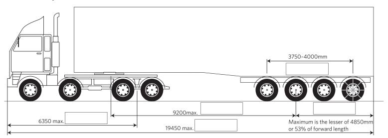
The information requested is required to confirm that the vehicle meets the dimension thresholds provided in Waka Kotahi NZ Transport Agencyapproved proforma designs for high productivity motor vehicles and to support an application for a High Productivity Motor Vehicle Permit under the Land Transport Rule: Vehicle Dimensions and Mass 2016.
