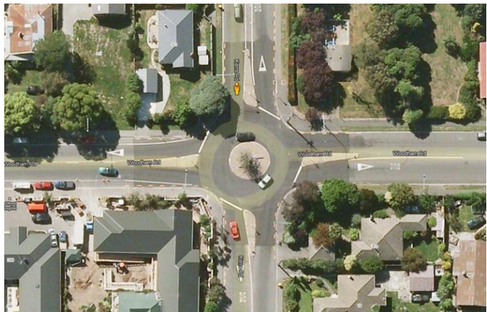
Photo 4–4: Example: Single lane urban roundabout. Source: Google Maps (2011)
