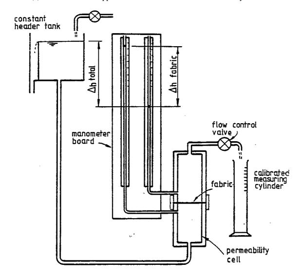
Figure A2: Filter Fabric Permeability Apparatus
