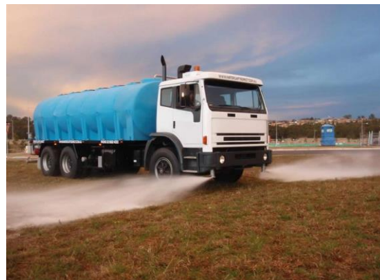
Dust suppression using a water cart
