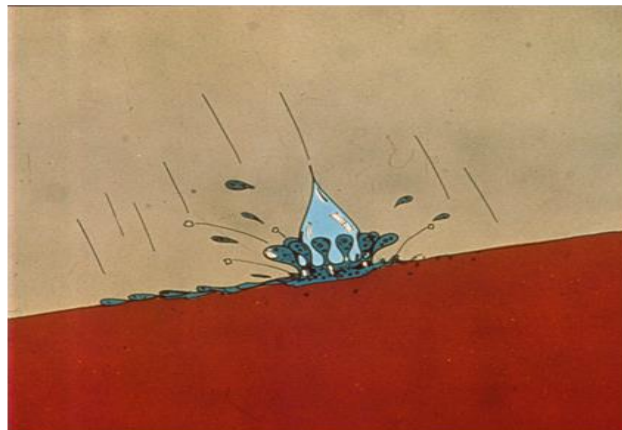
Schematic of Raindrop Splash
