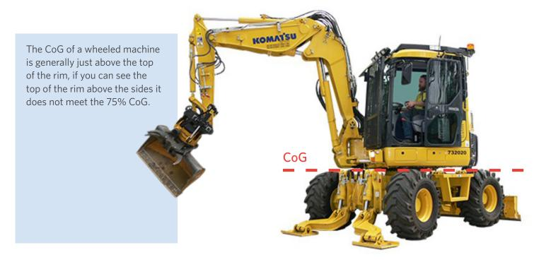
Note; the vehicle must also be capable of safely transporting the machine, commonly machines can show their weight in the model designation ie a 45, 450 or 4500 model will generally be 4500kgs and 15, 150 or 1500 is 1500kgs etc
