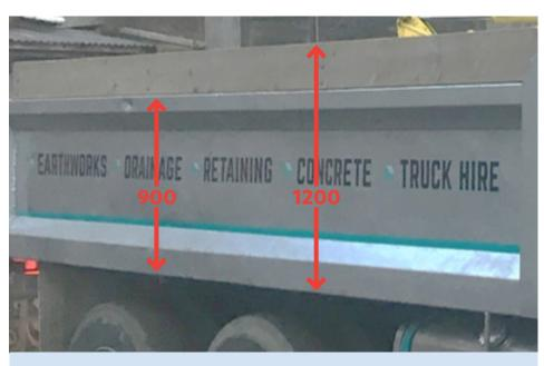
The Centre of Gravity (CoG) of the machine should be no higher than 75% of the sides, headboard and tailgate eg if the sideboard is 1.2mtr, CoG needs to be no higher than 900mm.
