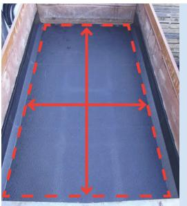
The digger must sit tight in the bin or within 100mm of the sides, front and rear so that it can't move around.
