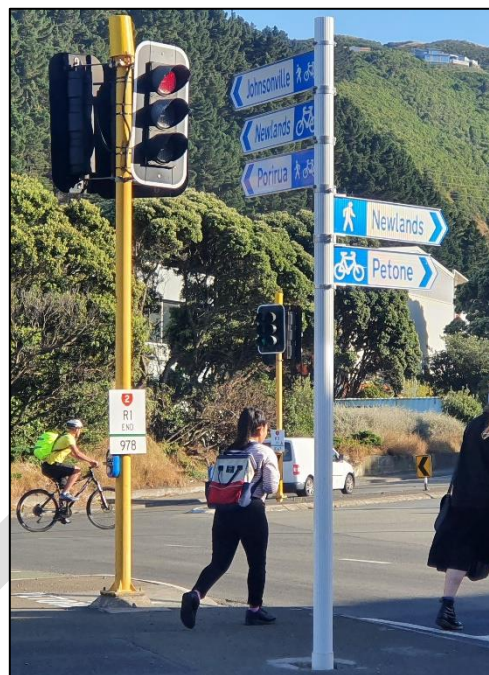
Figure 5: Cycle route intersection direction sign (with example installation on the right)
