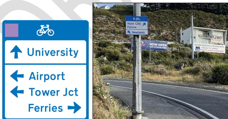
Figure 3: Advance direction signs for primary cycle routes (with example installation on the right)
