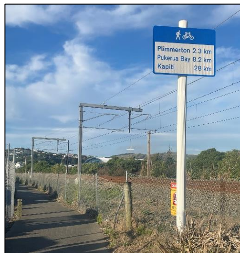
Figure 8: Confirmation direction sign (with example installation on the right)
