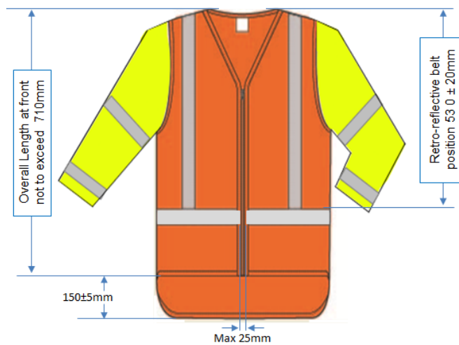
Figure 2B: Optional MTC sleeve for Stop/Go operator (100-105cm test size)
