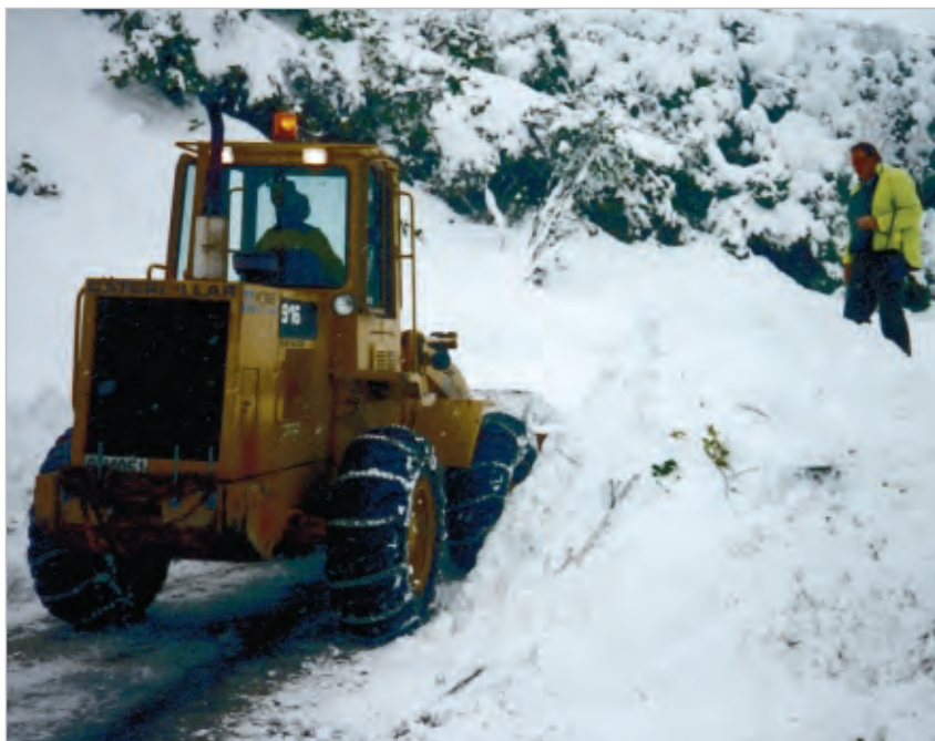
Figure 6-16 Snow clearing with graders and loaders (with wheel chains) can cause damage to the chipseal. Photo courtesy of Les McKenzie, Opus
