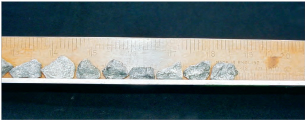
Figure 8-28 AGD (Average Greatest Dimension) apparatus. Photo courtesy of Joanna Towler, Transit NZ
