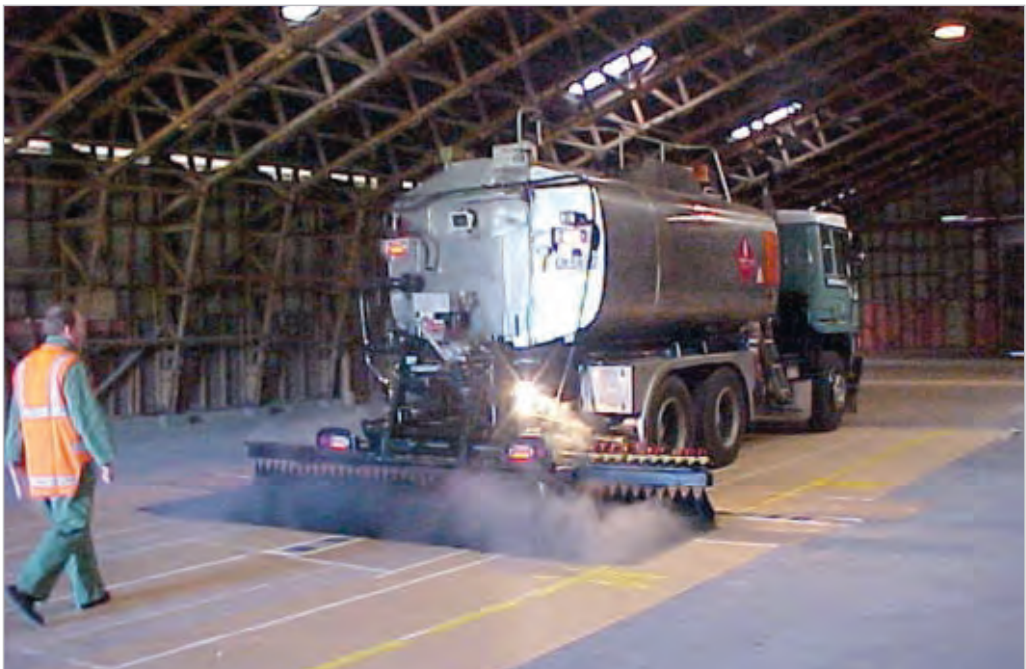
Figure 10-12 Calibration of bitumen distributor. Photo courtesy of Bryan Pidwerbesky, Fulton Hogan Ltd
