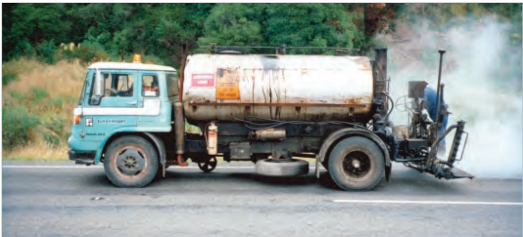
Figure 1-6 An old-style bitumen distributor (sprayer). Note the tall handle behind the distributor tank which was used to open and shut the spraybar. Photo courtesy of Laurence Harrow, Opus
