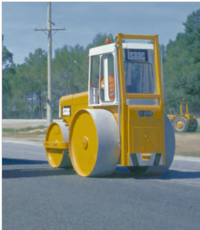
Figure 10-23 A steel-wheeled roller.
