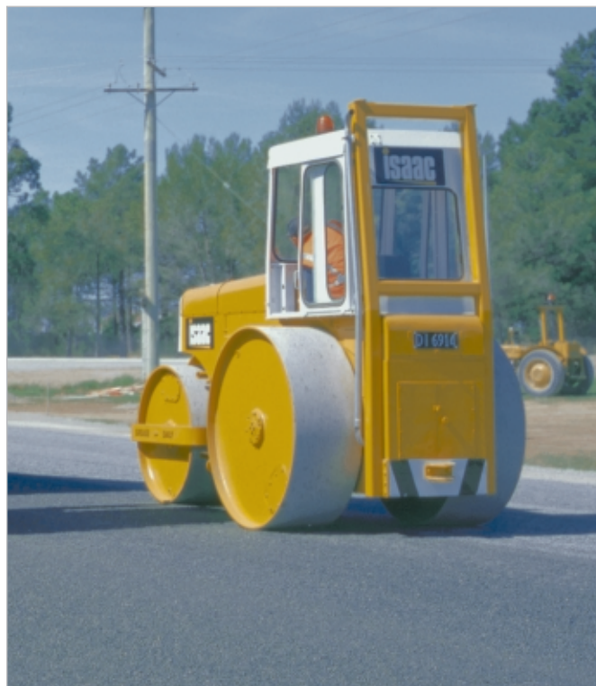
Figure 10-23 A steel-wheeled roller.
