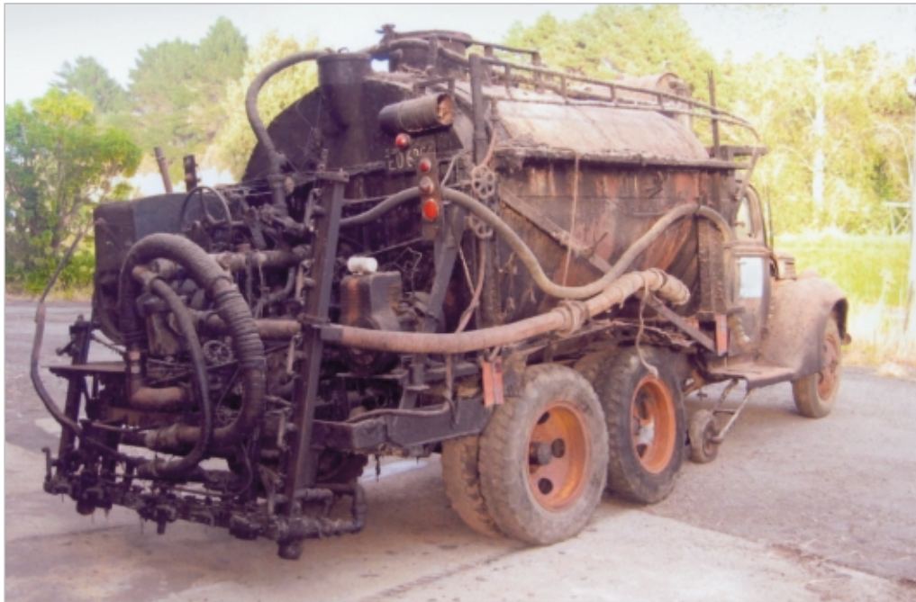
Figure 10-9 A bitumen distributor with an old-style lever-operated spraybar.
