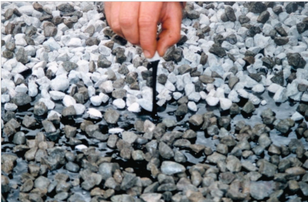
Figure 8-19 Removing a chip from a PMB chipseal reveals a long string of binder with enhanced elasticity. Photo courtesy of Les McKenzie, Opus
