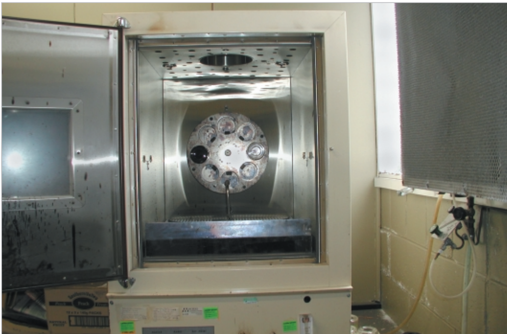
Figure 8-4 RTFO test apparatus used to simulate hardening in a chipseal.
