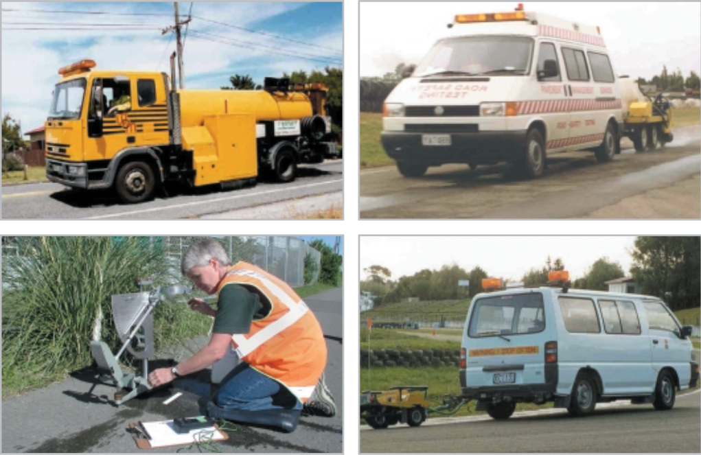
Figure 4-22 Machines used in New Zealand for measuring skid resistance. Clockwise from top left: SCRIM. Top right: RoAR. Bottom right: GripTester.
