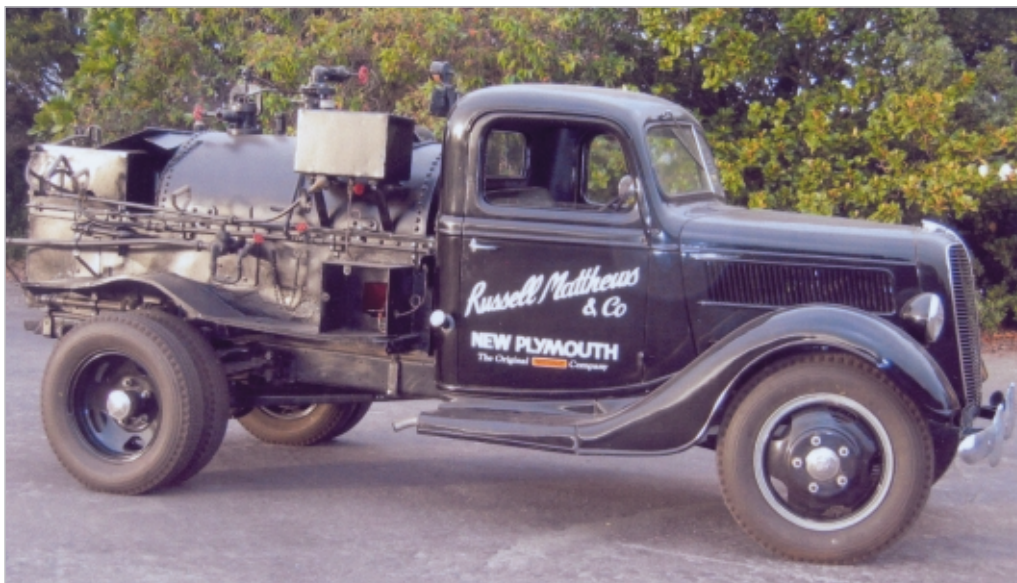
Figure 1-7 A 1940s bitumen distributor and hand sprayer, vacuum-filled and pressure discharged, on display at the property of John Matthews, Technix Group Ltd, New Plymouth.
