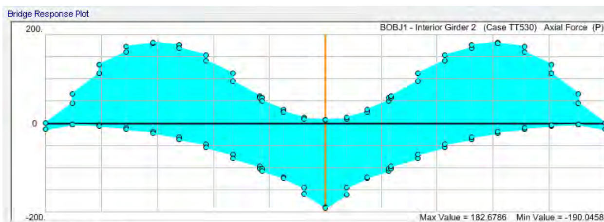
Figure C4A.4: Interior girder axial force envelope for TT530 in lane 1 (kN)
