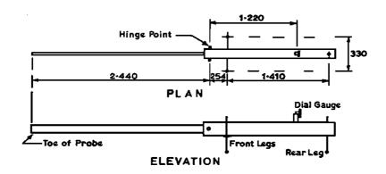
Fig 1. Diagram showing critical dimensions of Benkelman Beam
