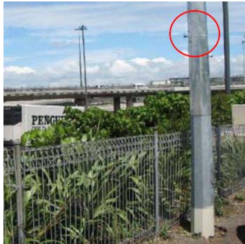
(b) a passive diffusion tube deployed at the central motorway junction, Auckland
