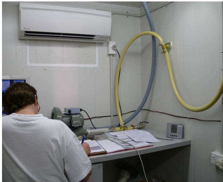
Figure 40: the sampling manifold inside the air quality trailer.
