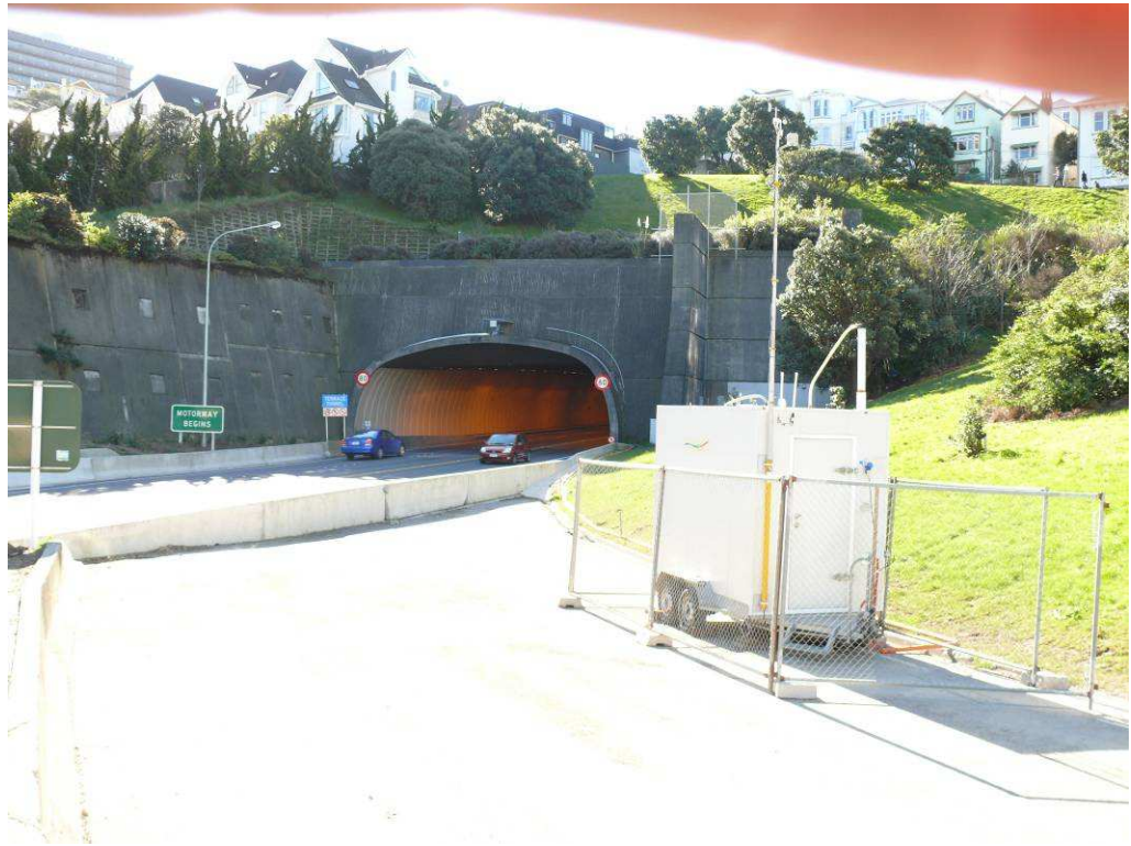
Figure 36: The air quality trailer at the southern portal of the Terrace Tunnel.
