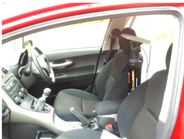
Figure 4.1 Sound level meter mounted between the front seats
