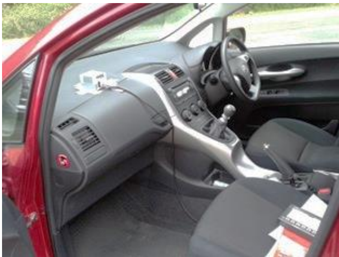
Figure B.1 Accelerometer mounted on the dashboard
