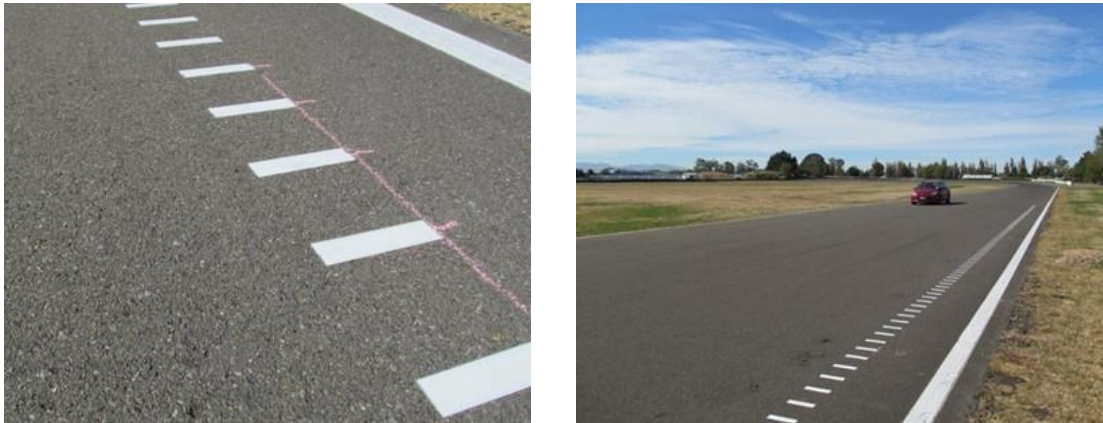
Figure 5.1 Line of polycarbonate strips at 250 mm spacing
