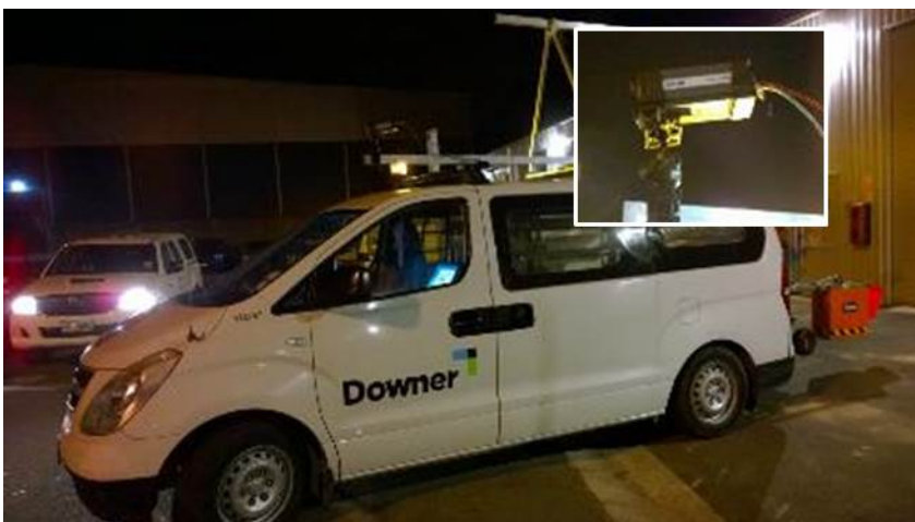
Figure 2.16 Installation of thermal camera in the survey vehicle
