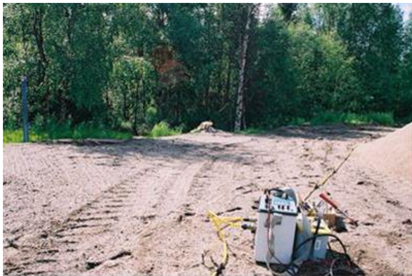
Figure A.27 Example of static multi- electrode array with IRIS Syscal unit
