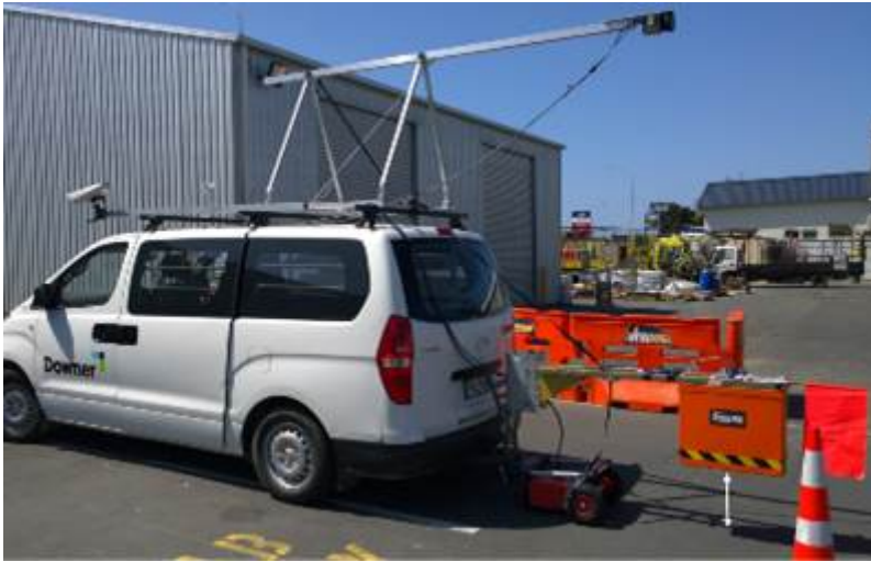
Figure 2.9 Antenna elevation analysis for roughness surveys (exact distance from antenna to pavement surface is measured continuously)
