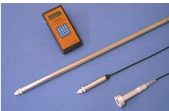
Figure A.14 Typical percometer sensors: the long tube probe is used for soil measurements, the short tube probe is installed inside the road structure and a surface probe is used to measure dielectric values and electrical conductivity from the material surface
