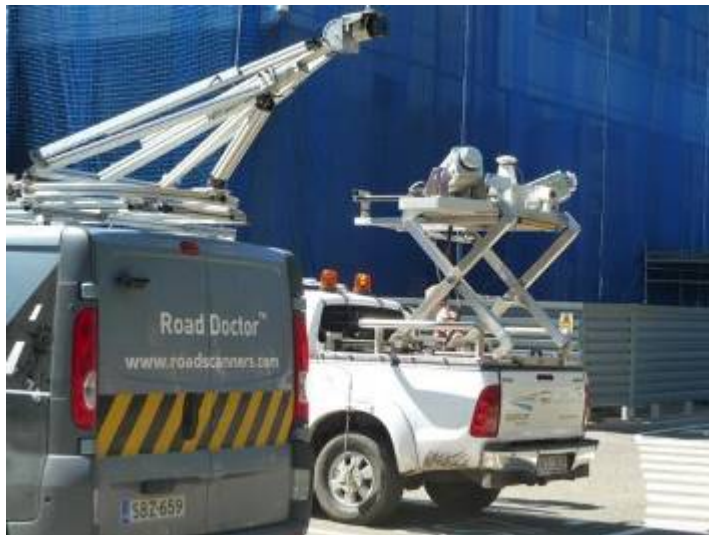
Figure A.61 2D (left) and 3D laser scanning systems (right) for road surveys
