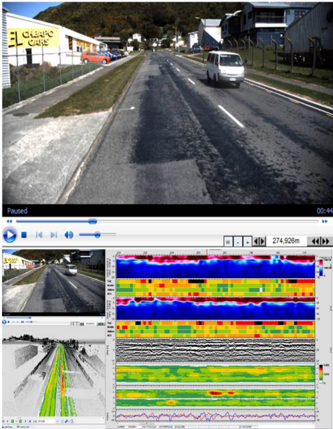
Figure B.10 High moisture locations at point 2 (274m) on Raiha Street in Porirua
