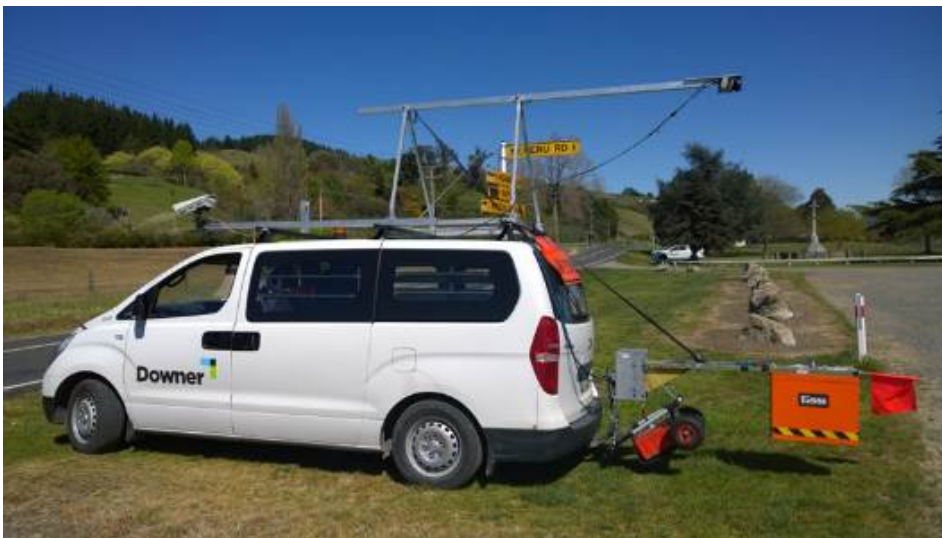
Figure 2.7 The survey van equipped with video camera (top front), laser scanner (high up), GPR ground coupled antenna (red box with wheels, elevated) and air coupled antenna (orange box far rear)
