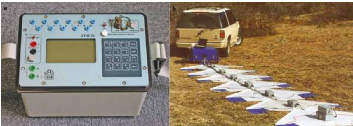
Figure A.57 (a) Electrical resistivity meter, (b) capacitive coupled carpets pulled on the surface behind a towing vehicle (source: IRIS Instruments)
