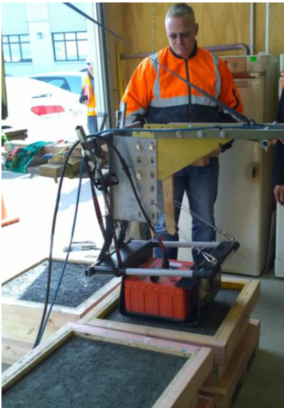
Figure 2.2 Performing 'box tests' in Downer laboratory in Auckland. In this case measurements are carried out using 400 MHz ground coupled antenna
