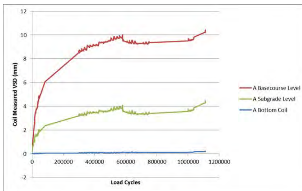
Figure C.3 Measured vertical surface deformation/rutting from CAPTIF strain coils for CAPTIF test 1A (6 tonne axle)
