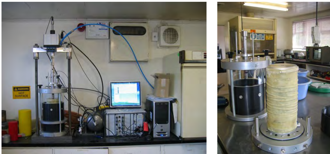
Figure 5.1 Repeated load triaxial apparatus
