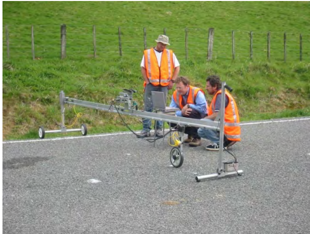
Figure 6.2 Rutting measurements on the New Zealand- LTPP Programme
