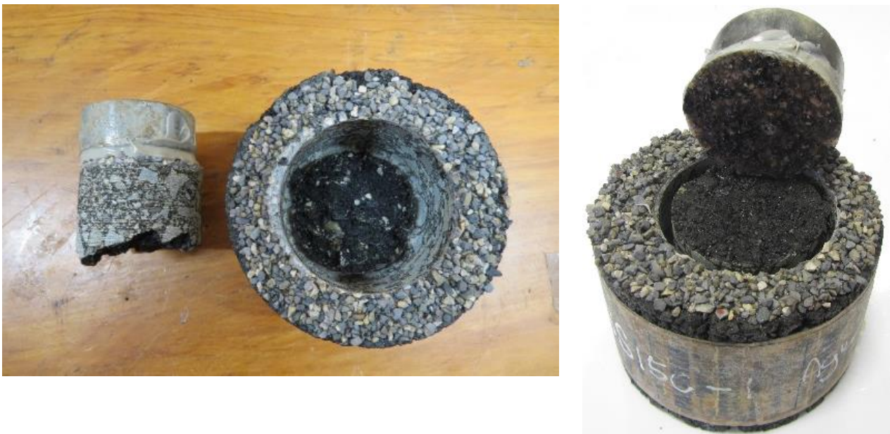
Figure 3.8 (Left) Cohesive failure in the mix 15 substrate versus; (right) adhesive failure of the specialist surfacing system after ageing for 40 days
