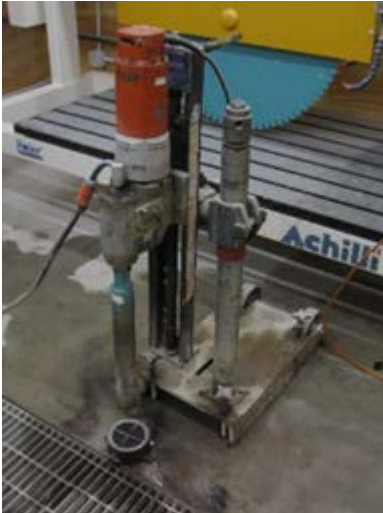
Figure A.4 Coring equipment and the test specimen setup
