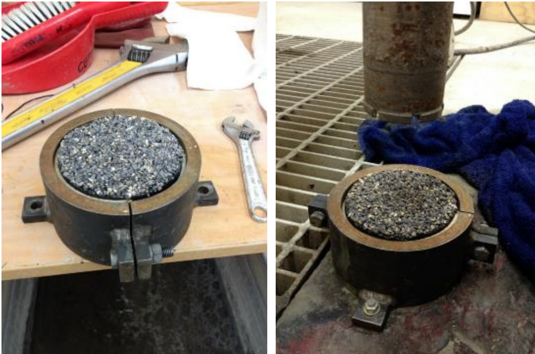
Figure 3.2 Example of an asphalt substrate with calcined bauxite system in preparation
