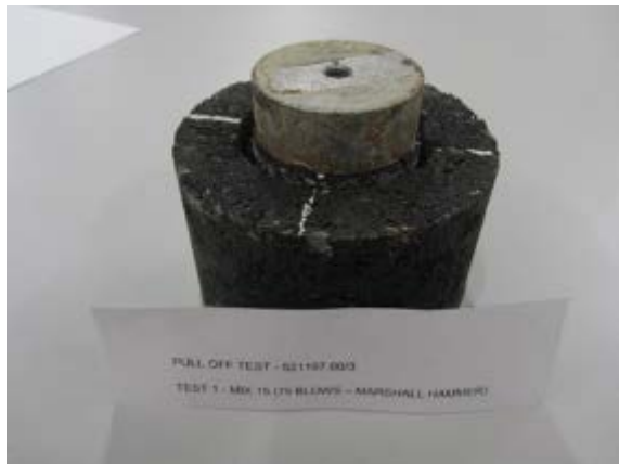
Figure A.6 Test specimen with aluminium disc attached
