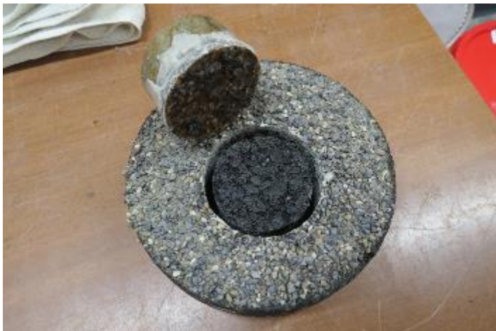
Figure 3.10 Example of an aged mix 20 core with an epoxy- based calcined bauxite system
