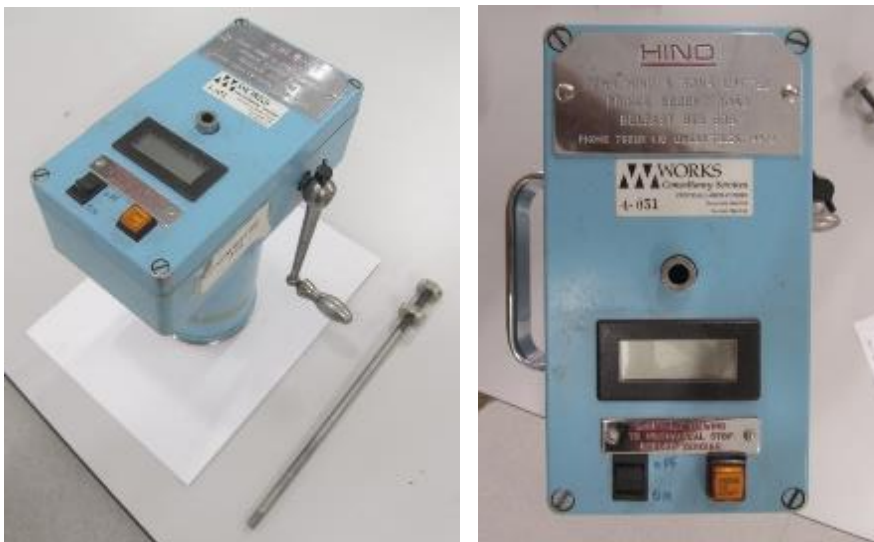
Figure 3.1 Illustrations of a pull-off bond tester
