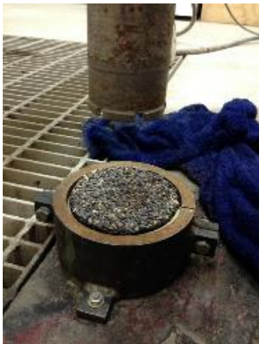
Figure A.3 Setup of a test specimen for coring cut
