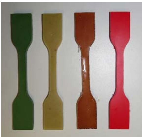
Figure 3.20 Examples of different types (D, A, C, B) of resin used in calcined bauxite systems in New Zealand
