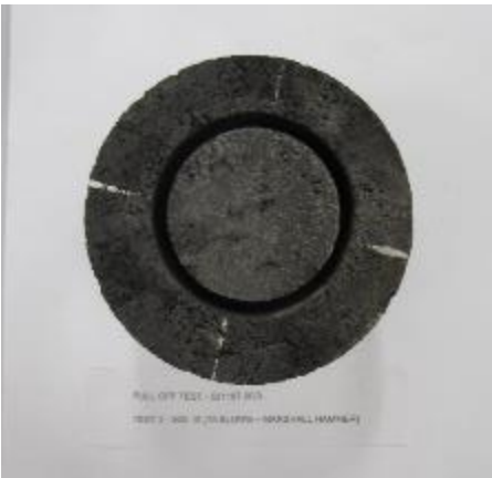
Figure A.5 Test specimen with a circular cut
