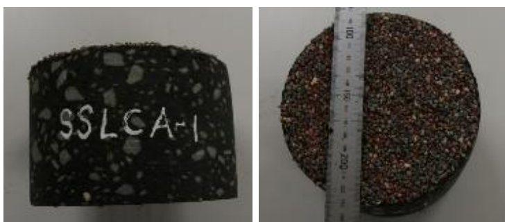
Figure 3.3 Illustration of a mix 20 asphalt sample cored from SH1 near Wellington and used as test substrate for a calcined bauxite system
