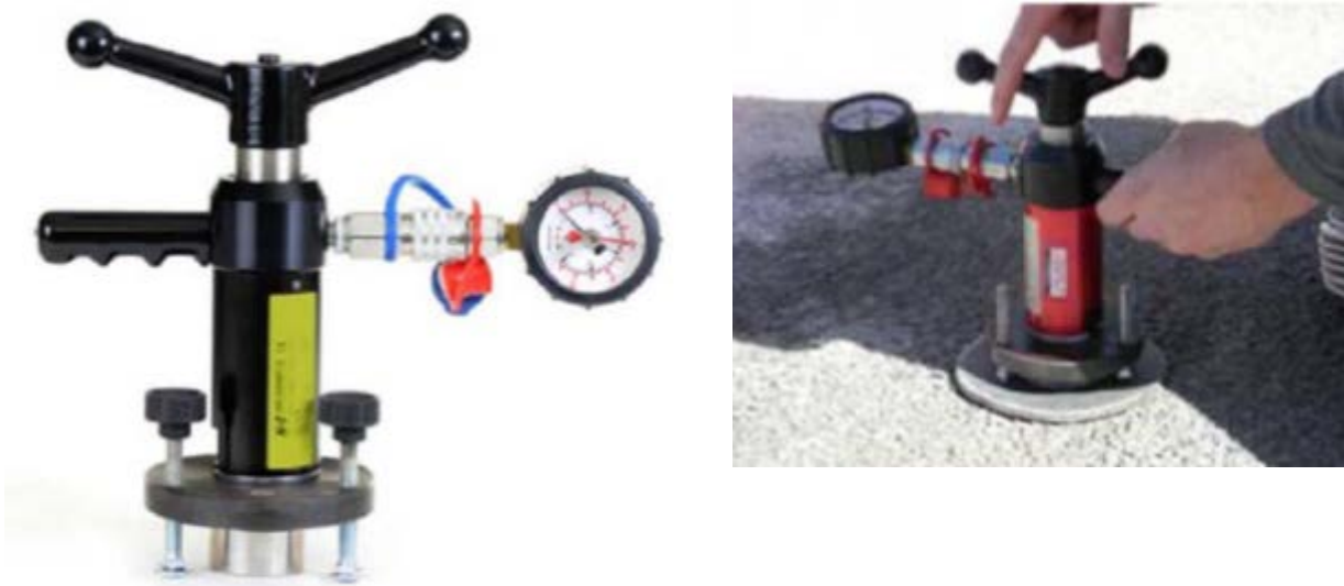
Figure 2.6 (Left) A pull-off bond test device; (right) the device in action
