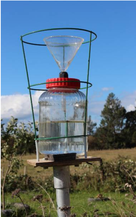
Figure 4.18 Dust deposition gauge
