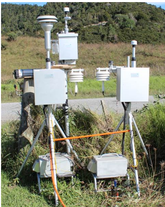
Figure 3.12 BAM TSP (left), BAM PM 10 (right) and Dustmote PM 10 (centre) installed at untreated north 5m site
