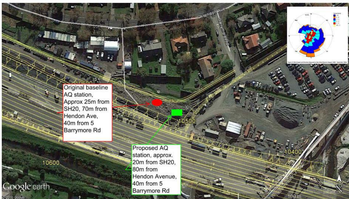
Figure 2: The proposed location of the southern air quality monitoring station
