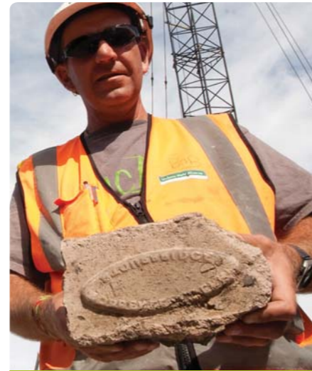
An old fire brick from Staffordshire in England was unearthed in Victoria Park. It would have been used in a kiln or furnace – possibly the former city destructor (now Victoria Park Market).
