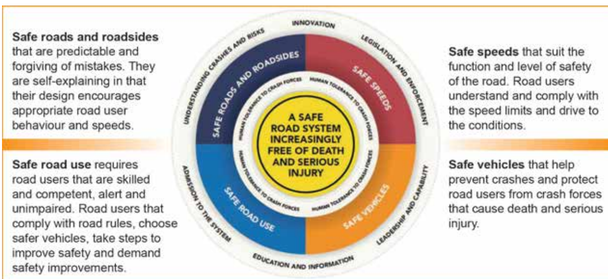
Figure 3.1 Safe System cornerstones
