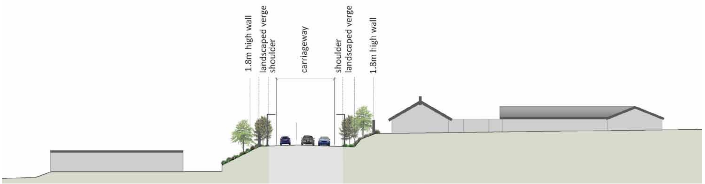
Figure 5.51: Waitangirua Link Road - Cross section C
