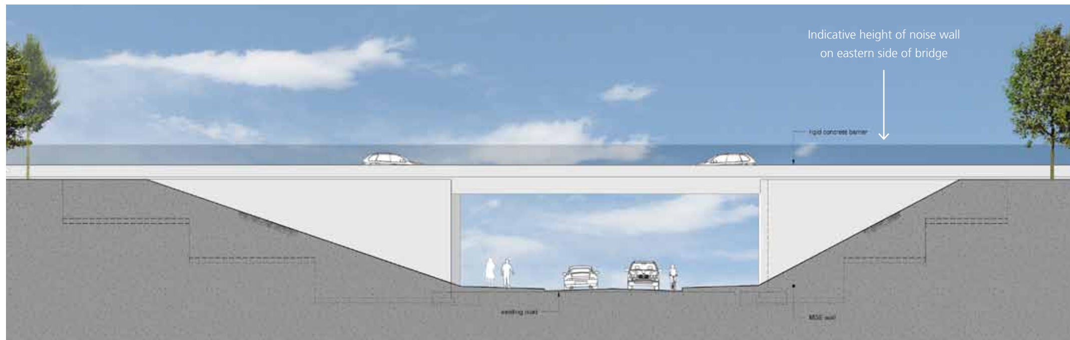
Figure 5.72: Bridge 26 Collins Avenue Bridge Elevation
