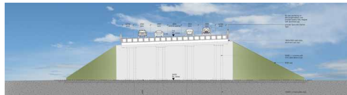
Figure 5.39: Bridges 13 & 14: SH58 Interchange cross section
