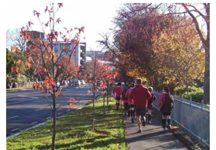
Photo 4.17: Footpath separated from road by grassed berm
