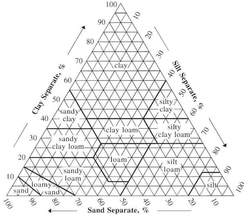
**Figure O3 - Saturated Hydraulic Conductivity Code Approximation**
