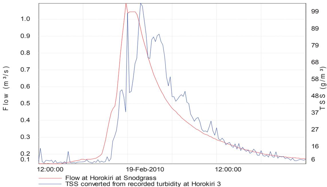
■ **Figure 15.90 Continuous TSS Data and Flow on the Horokiri Stream During a Rainfall Event on 18 and 19 February 2010**
