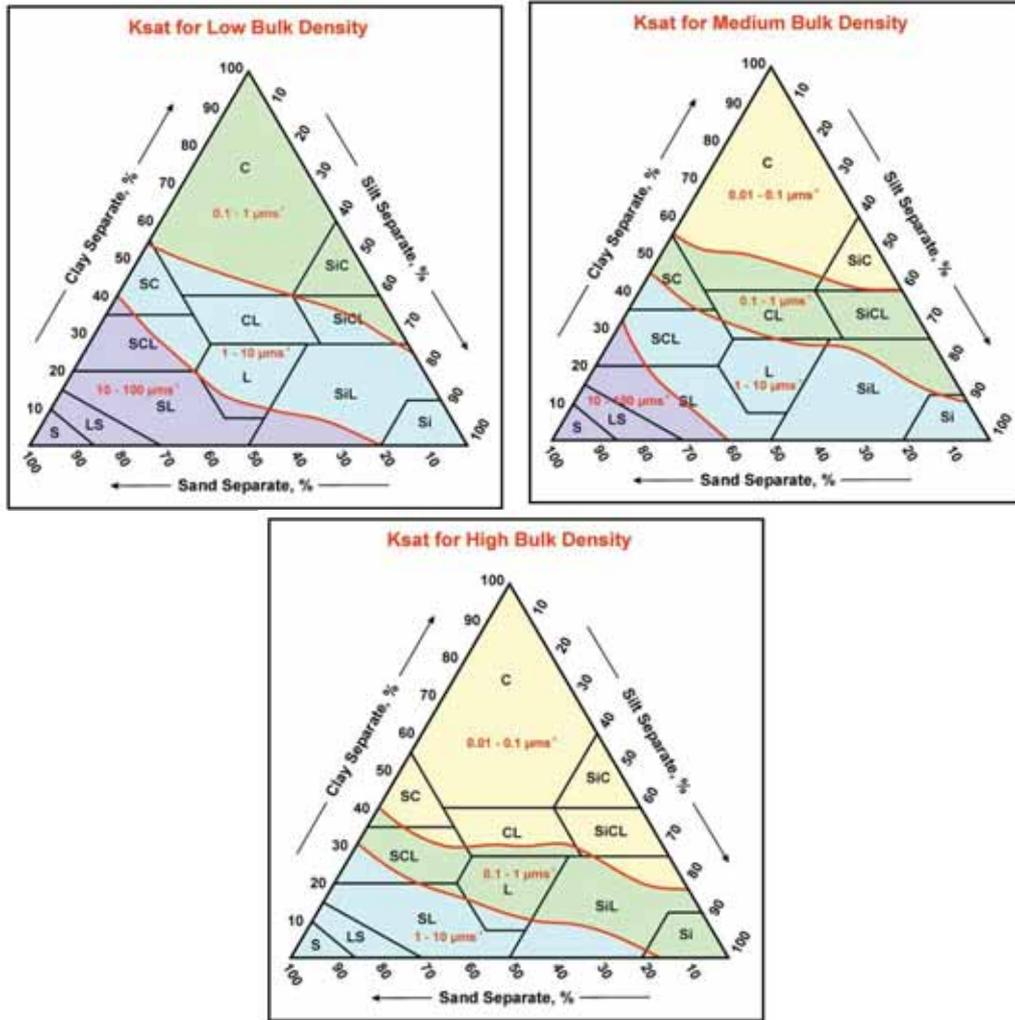
**Figure O2 Saturated Hydraulic Conductivity**
