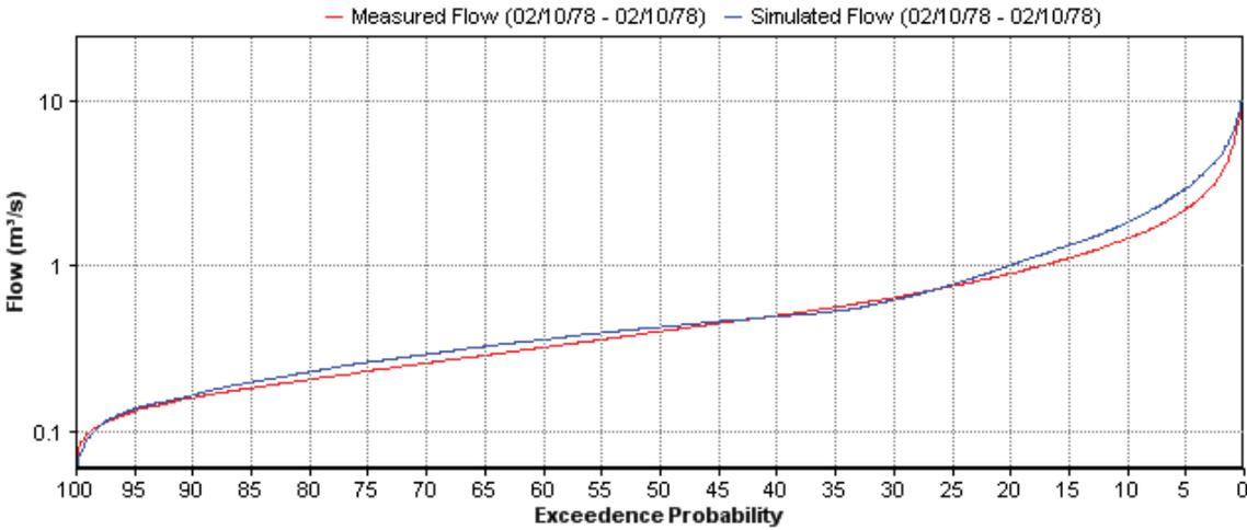
**Figure K.6 Pauatahanui Stream: Observed and Simulated Flow Duration Curves**
