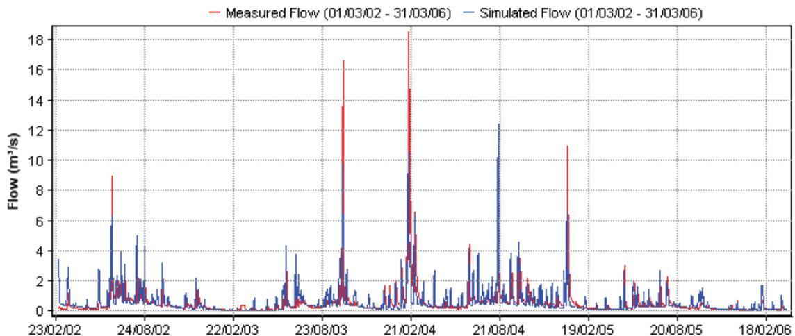
**Figure K.4 Horokiri Stream: Observed and Simulated Hydrographs**
