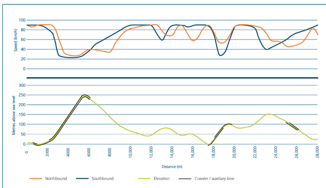
Figure 7.1: Longitudinal profile of the Main Alignment showing the predicted heavy vehicle travel speeds and the location of crawler / auxiliary lanes
