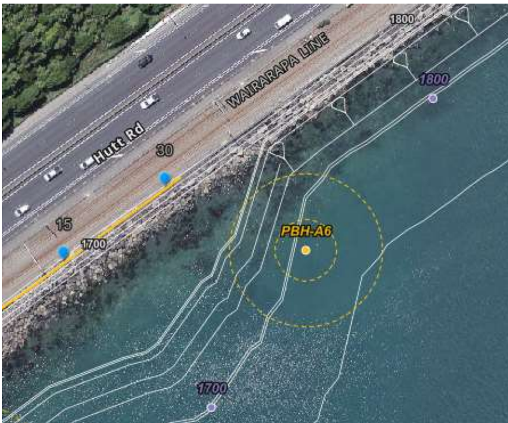
Figure 6. Example of modelled 75 dB L_{Aeq(15\ min)} noise contours for borehole (yellow dot) geotechnic investigations. Outer yellow dotted line based on no noise mitigation, inner yellow dotted line with noise mitigation measures. Penguin habitat identified by yellow solid line on revetment and penguin burrows by blue numbered dots
