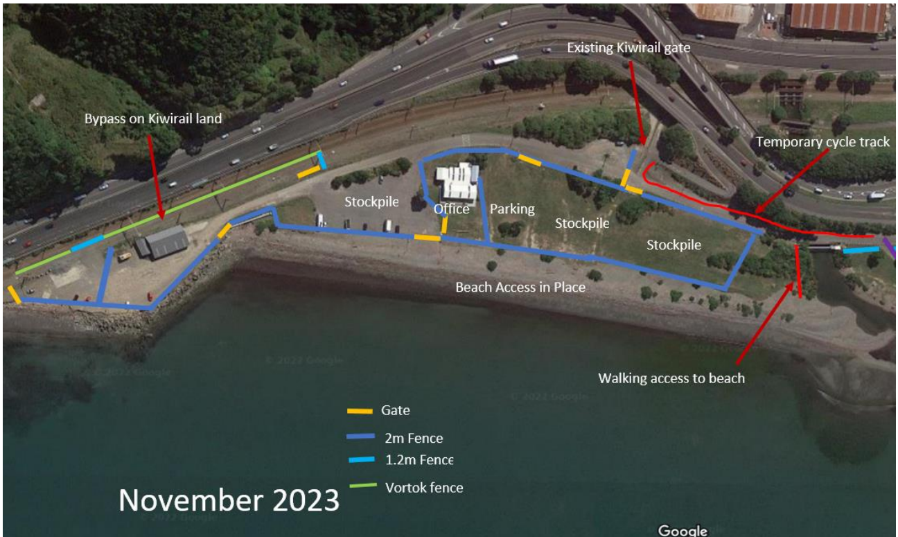
Figure 5.3. Site layout of the Pito-One Construction Yard (western side of Honiana Te Puni Reserve)
