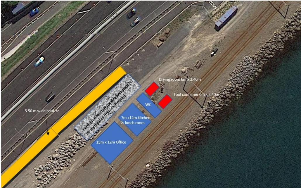
Figure 5.2. Site layout of the Ngā Ūranga Construction Yard
