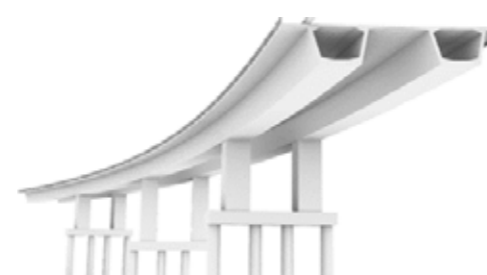
Twin cast box girder balance cantilever options.
