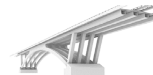
Single span Steel Arch.
