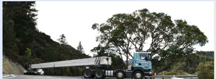
One of Taipā's beams lining up to cross Kaeo Bridge. The rear, independent unit is called a jinker and is remote controlled. The jinker operator travels in one of the pilot vehicles and swings into action when the front tractor unit operator requires assistance to get around tight corners.
