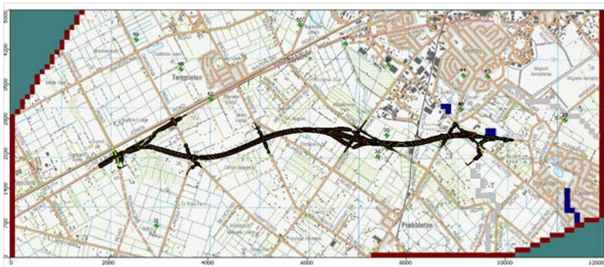
Figure A1 Regional Model Set-Up Showing Inactive Cells, Constant-Head Boundaries Rivers and Drains
