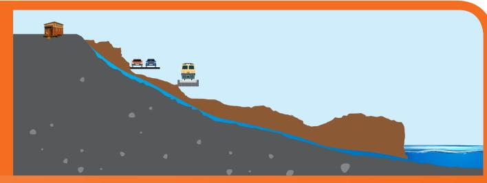
We have removed the weight from the top of the slip, redirected the water and installed monitoring wells
