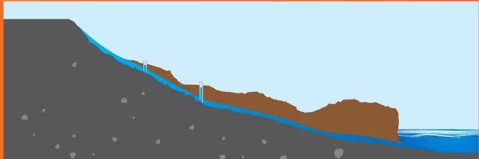
We are installing drains to take the water out of the slip
