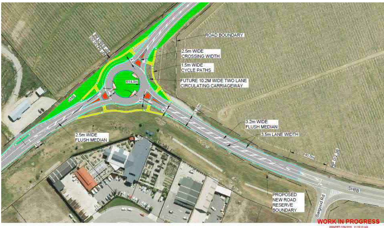
Figure 1: Proposed improvement to SH6/SH8B intersection
