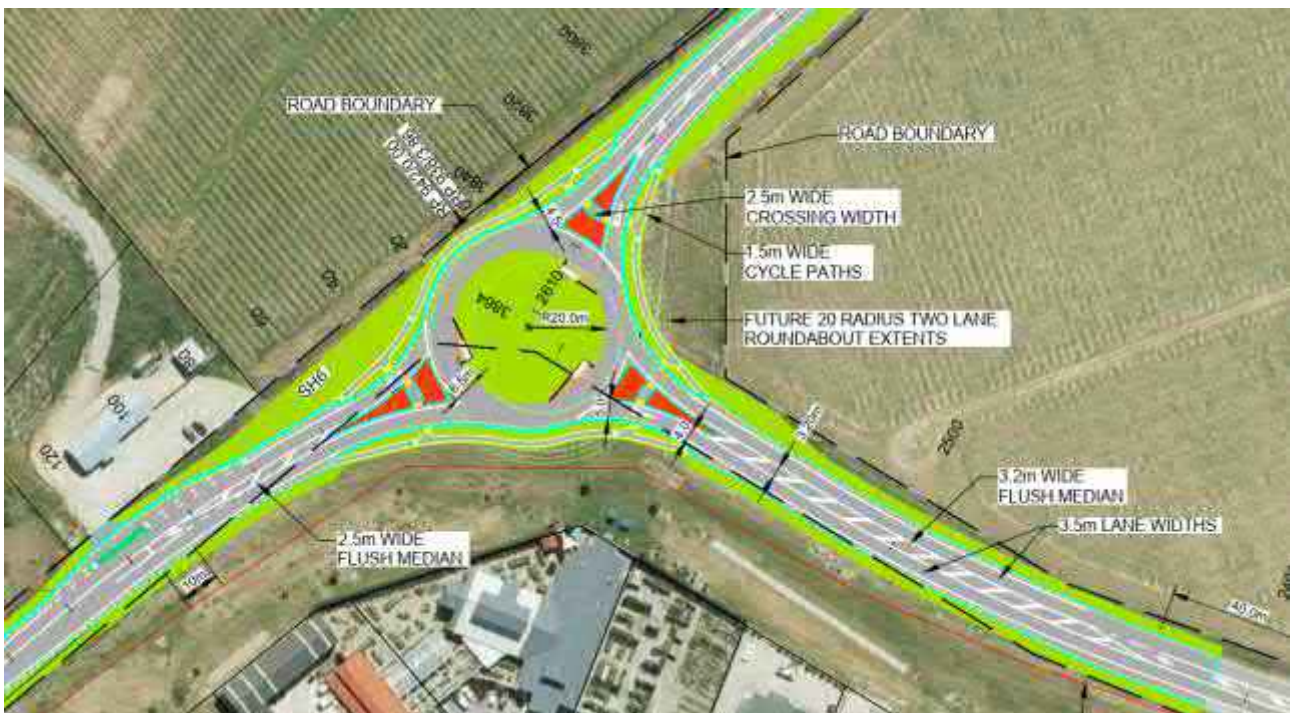
Figure 1: Proposed improvement to SH6/SH8B intersection - 20m radius island
