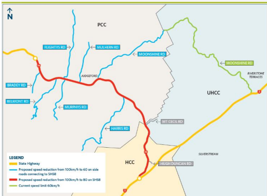
Diagram showing where speeds would be reduced to 80km/h on SH 58 and council roads connecting to SH58.
