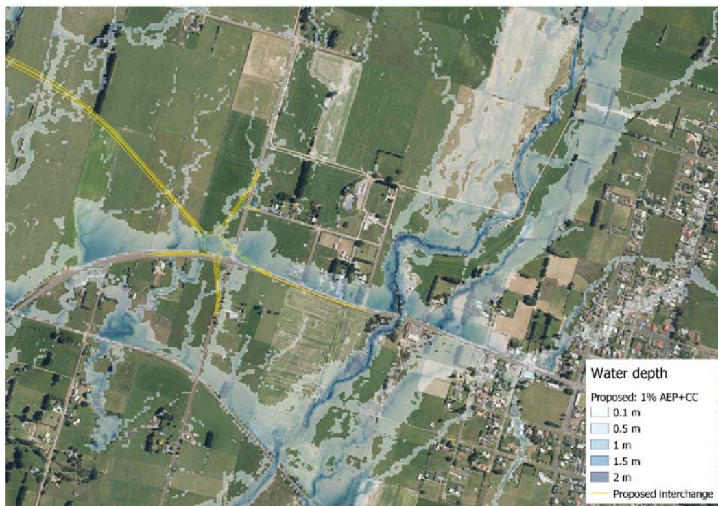
Figure D.67: Overland flow paths and flooding during a 1% AEP 6-hr design rainstorm (increased to allow for the potential effects of climate change to 2120) with the existing terrain. The location of the proposed roundabout following construction is shown by the dotted outline.
