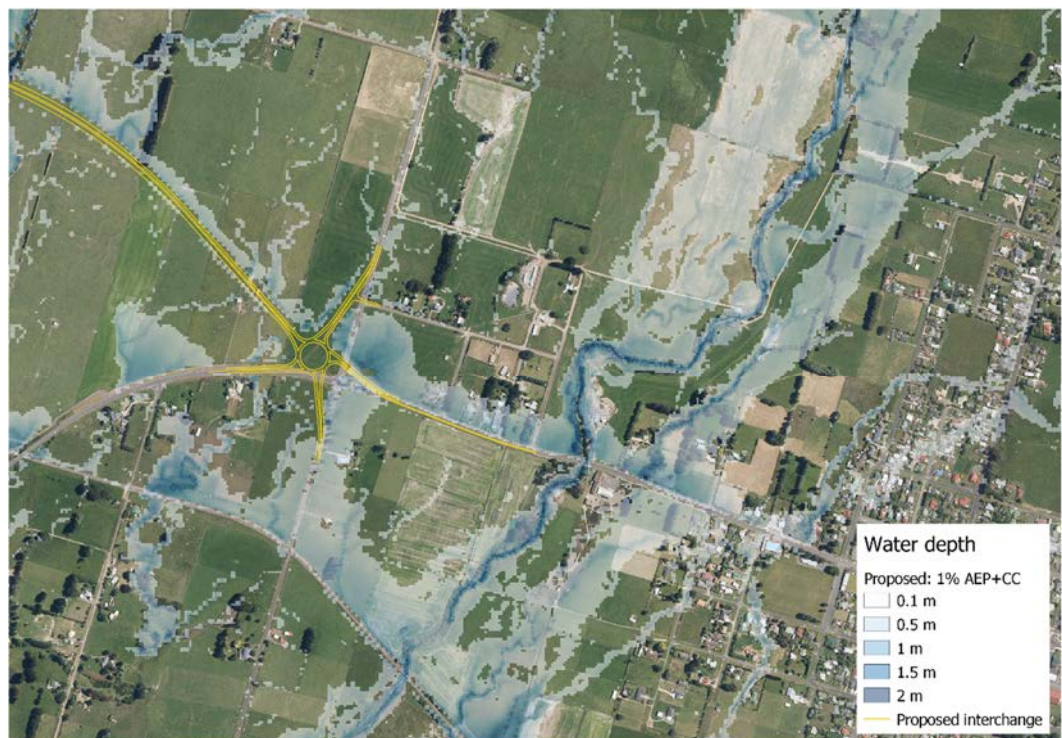
Figure D.68: Overland flow paths and flooding during a 1% AEP 6-hr design rainstorm (increased to allow for the potential effects of climate change to 2120) following construction of the roundabout which is shown.
