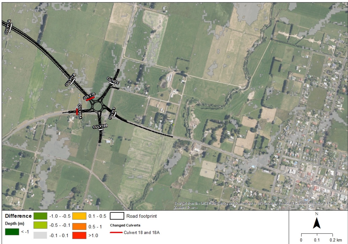
Figure 5: Differences between installing box culverts and circular culverts for Culverts 18 and 18A.
