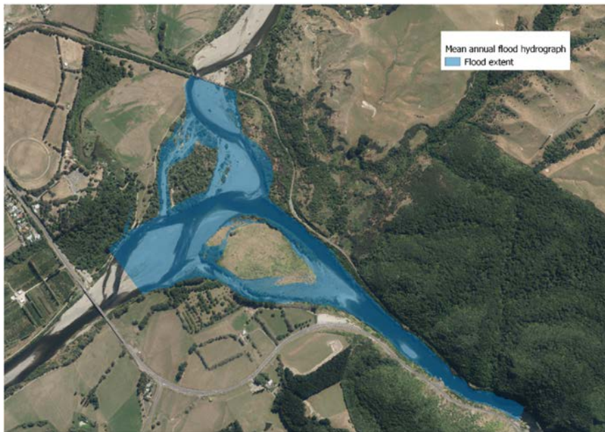
Figure D.39: Extent of inundation during a mean annual flood in the Manawatū River and hence the active channel under the existing environment.
