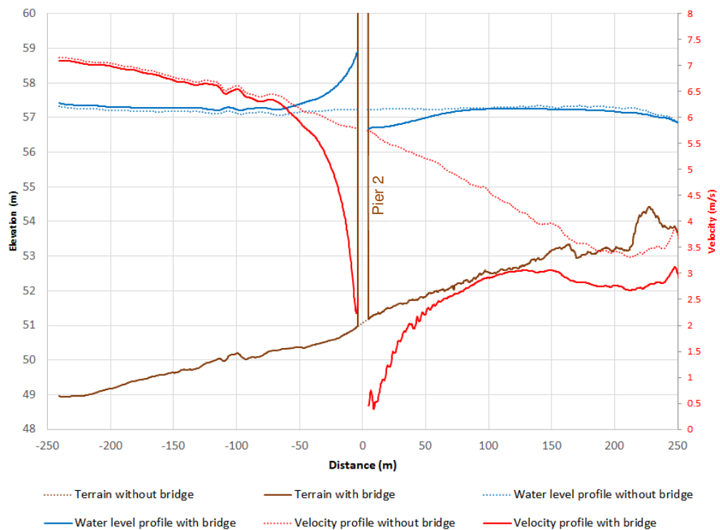
Figure D.50: Changes in water level and velocity as a result of construction of Pier 2 and the Manawatū River Bridge (BR02).
