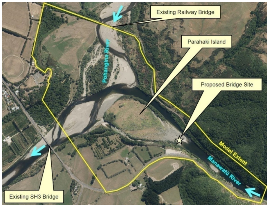
Figure D.38: Extent and bathymetry of the 2D model of the Manawatū River.
