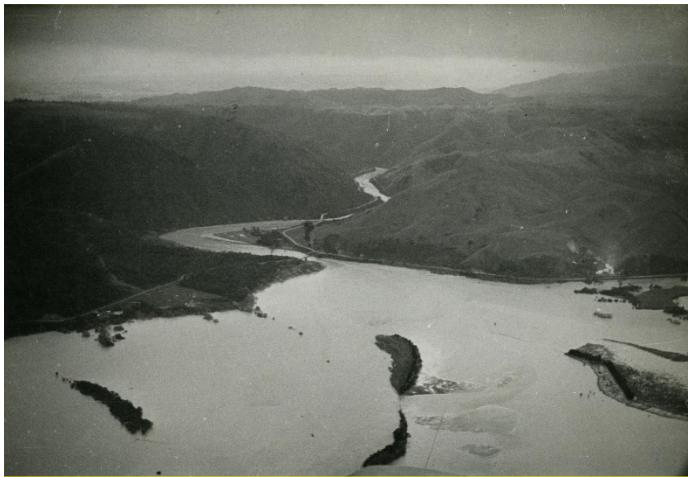
Figure D.71: Backwater flooding upstream of the Gorge during the 5 May 1941 event.
