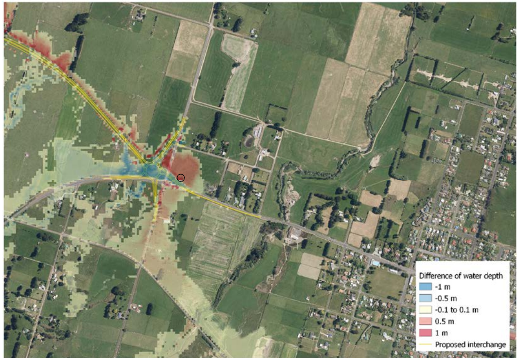
Figure D.69: Differences in the depth of flooding during a 1% AEP 6-hr design rainstorm (increased to allow for the potential effects of climate change to 2120) following construction of the roundabout, which is shown. The black circle shows the location used for determining the duration of inundation.
