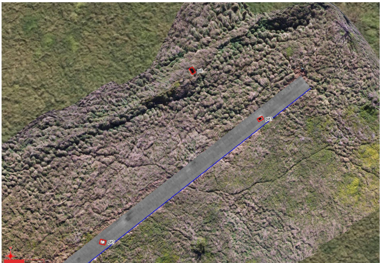
Figure 18: Area of the observed pit and possible pits indicated by the geomagnetic survey. Clearly visible is the 'quiet' background of the geomagnetic survey indicating top soil rather than gravel layers.
