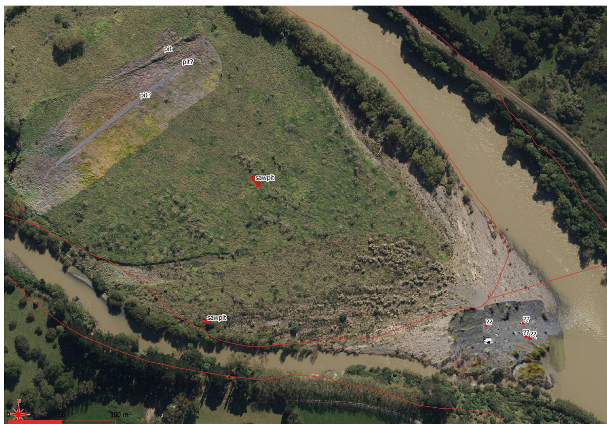
Figure 12: Features and indicative features from the walkover and from the geomagnetic survey. The picture also shows the geomagnetic survey areas surrounded by the high resolution ortho photos from the UAV survey.
