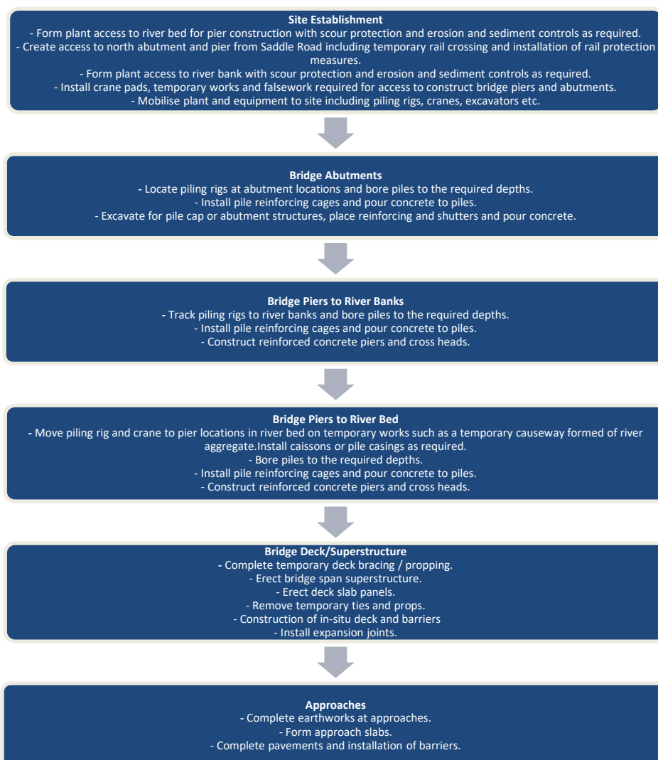
Figure 18 – Possible Bridge Construction Methodology
