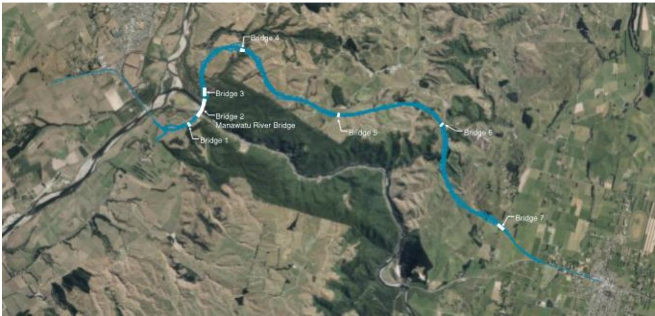
Figure 1: Indicative main alignment and potential bridge locations
