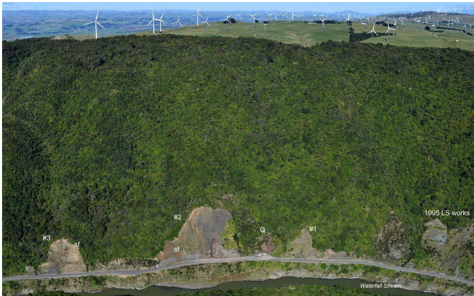
Figure 10. Oblique aerial photo of the central section of the Manawatu Gorge from ~RP491/0.60–1.30 showing the area of the 1995 landslide works, the „Quarry“ where small landslides occurred in 1940 and the 1960s, and three of the largest landslides (#1, #2, and #3) which occurred during the February 2004 rainstorm. The largest failure (#2) closed SH3 for over two months. Small failures ( sf ) have occurred on the scars of landslides #2 and #3 in the last 12 months.
