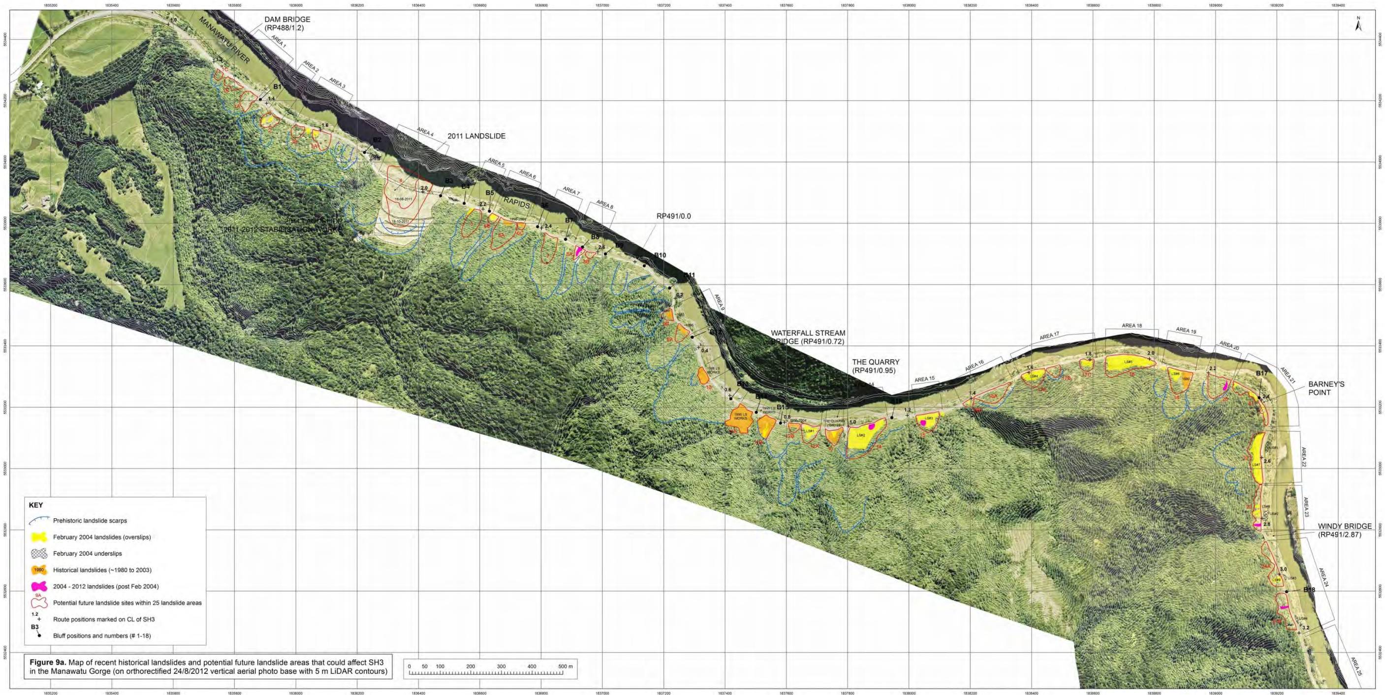
Figure 9a. Map of recent historical landslides and potential future landslide areas that could affect SH3 in the Manawatu Gorge (plotted on base of vertical aerial photos taken on 24 August 2012, with 5 m LiDAR contours).
