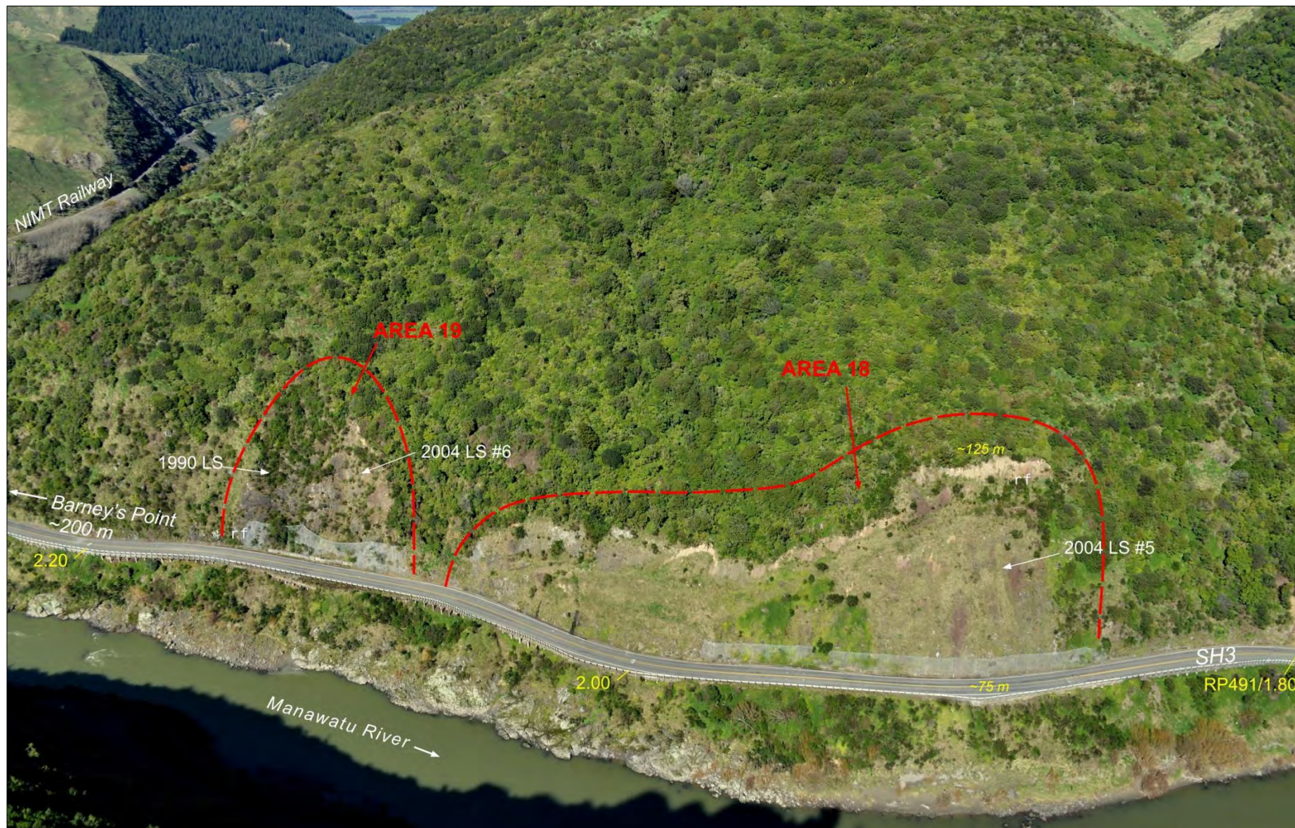
Figure 18. Aerial view of potential landslide Areas 18 and 19 and the sites of landslides which closed SH3 in 1990 and 2004 (#5 and #6) between RP491/1.80 and 491/2.20, about 200 m downstream of Barney's Point. The small recent failure ( rf ) on the head scarp of the 2004 landslide #5 suggests that Area 18 is perhaps more vulnerable to future failures than Area 19. The potential for failures at these sites is slightly less than those in the centre of the gorge.
