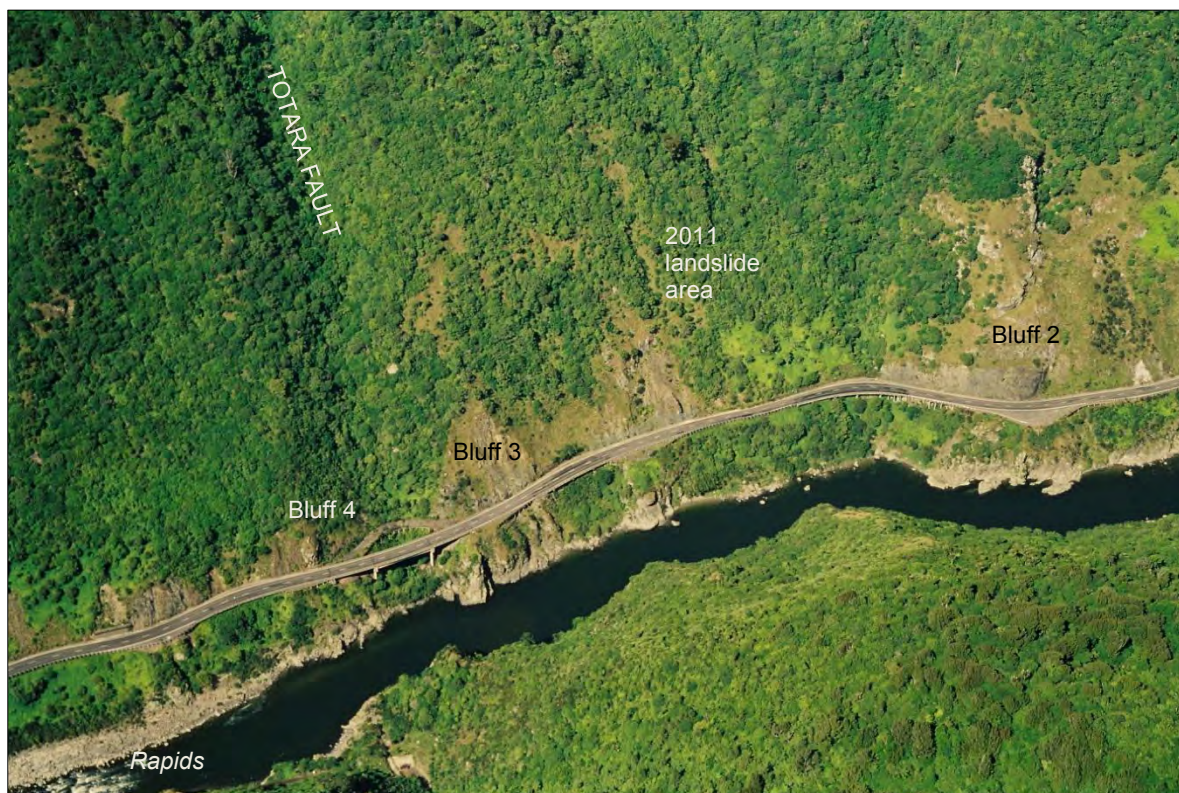
Figure 12. January 2000 photo of the 2011 landslide area, which developed on a slope underlain by thick colluvium deposits between bluffs of strong sandstone (B2, B3) in the Manawatu Gorge. The lower part of 2011 landslide area is sparsely vegetated because of shallow failures 1930-1940 and 1968-69 (compare with Figures 8 and 23).
