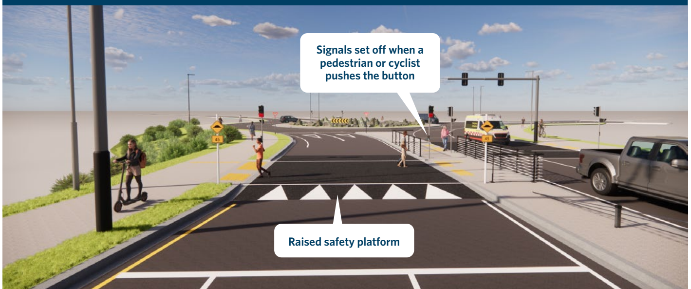
Visualisation of the signalised crossing on raised safety platform at the new roundabout at Coatesville-Riverhead Hwy
