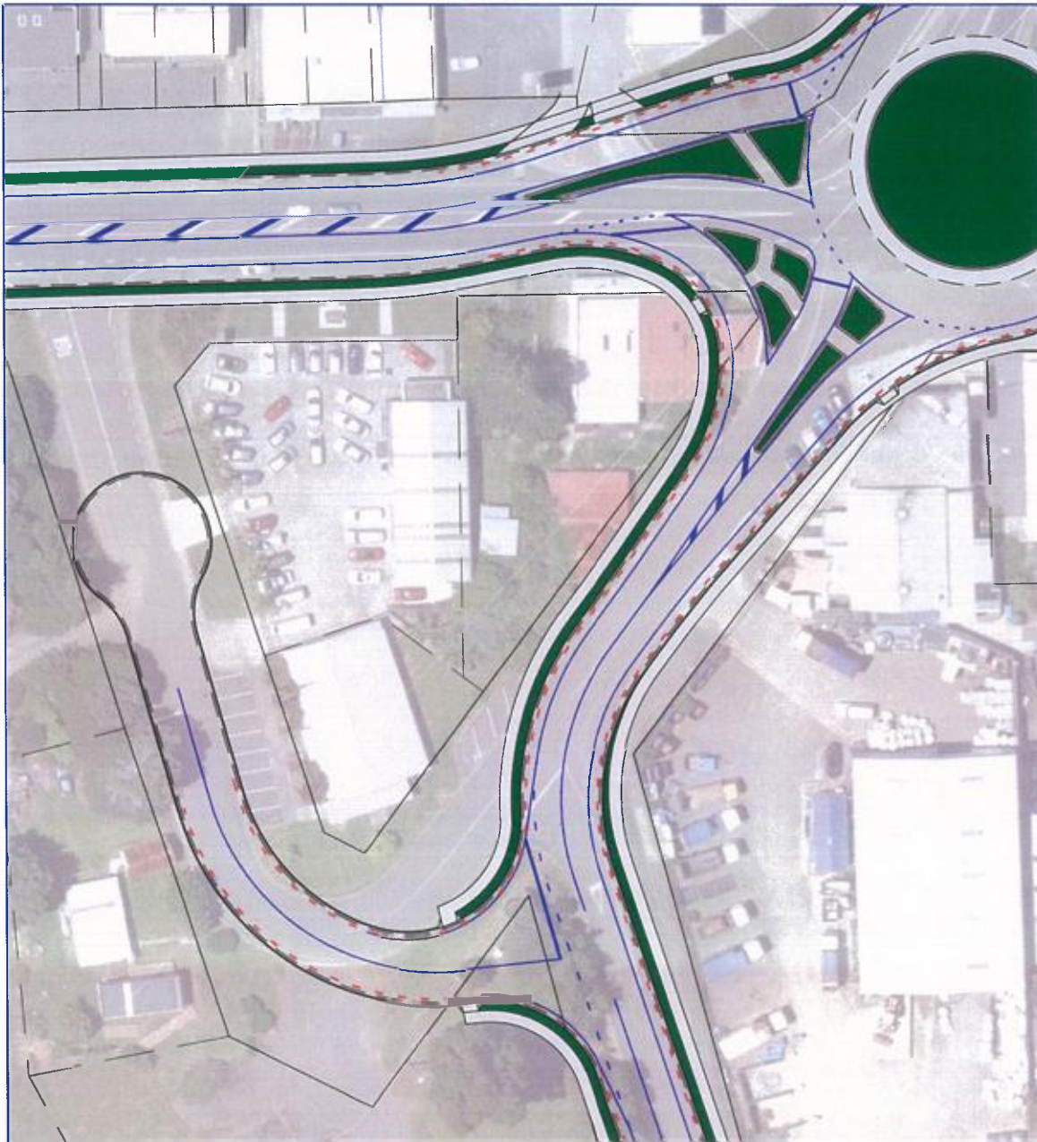
Figure 6: The proposed closure of the northern intersection of Waipapa Loop Road with SH10, with a cul-de-sac treatment.
