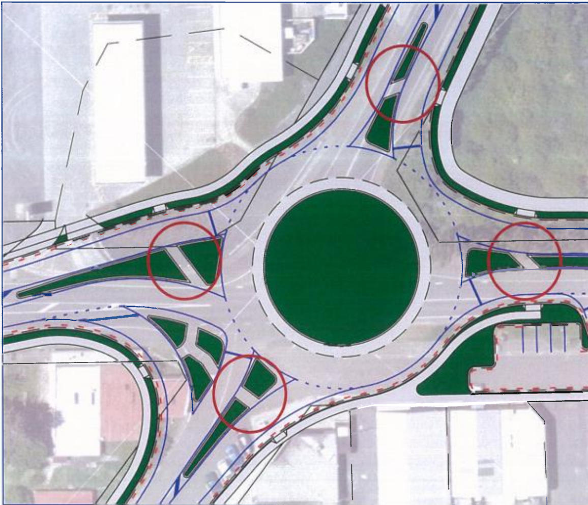
Figure 5: The crossing points within the entry islands are not perpendicular to the opposite crossing points.
