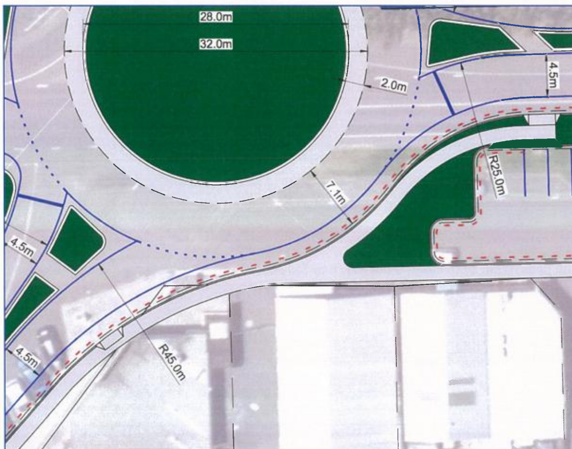
Figure 11: The footpath is next to the road through the left turn from SH10 into Waipapa Loop Road.
