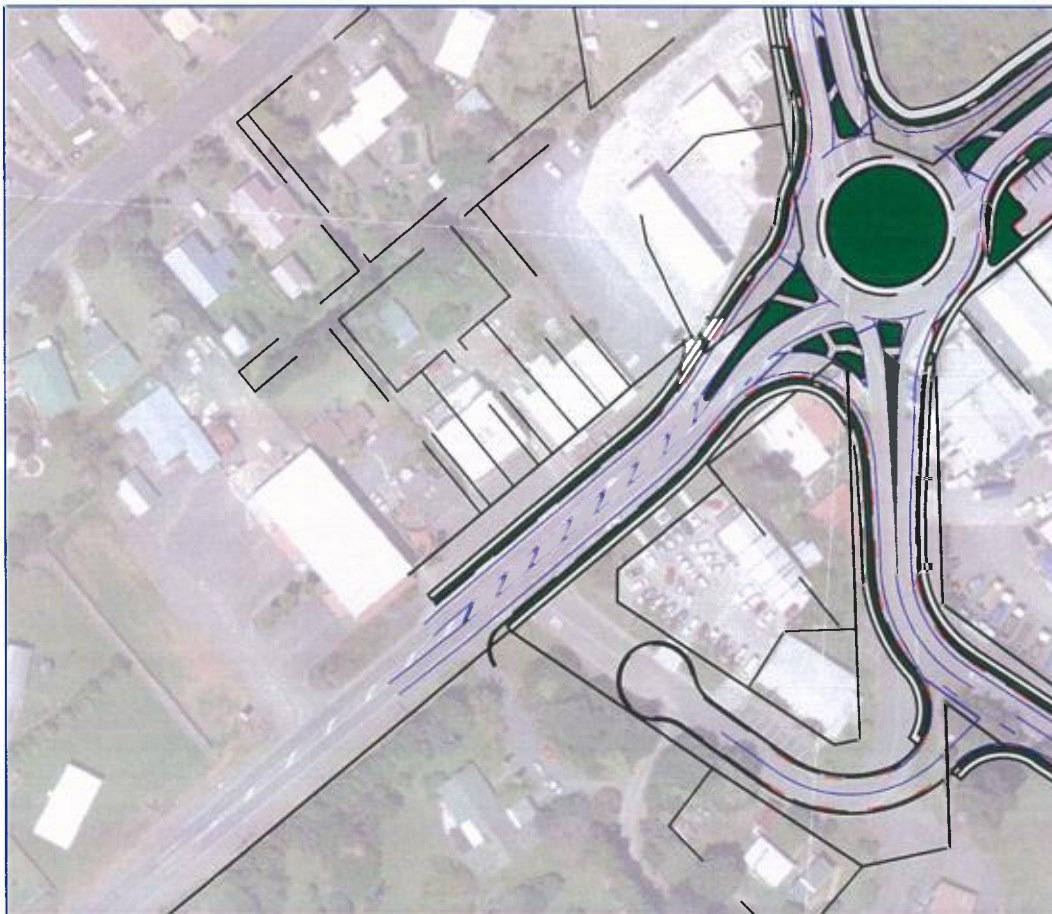
Figure 17: The SH10 north approach to the roundabout tie-ins to the existing central flush median treatment.
