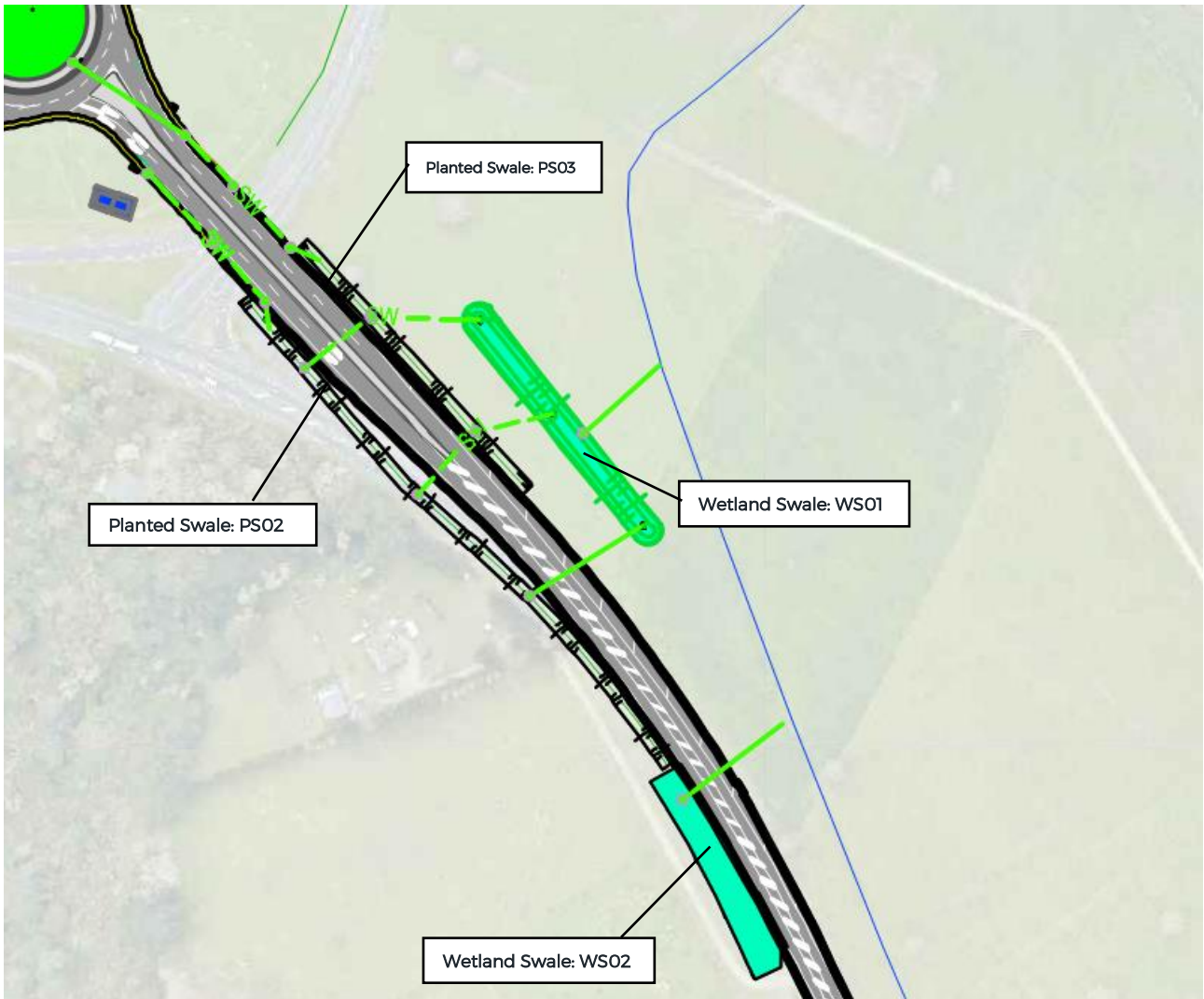
Figure 4-6: Tirau Leg - proposed stormwater design
