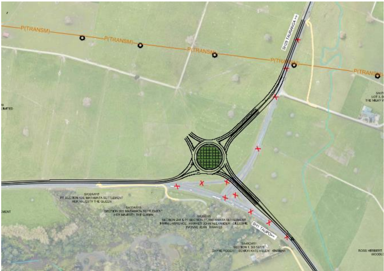
Figure 6-1: Recommended Option C - The proposed roundabout on the western side of SH29
